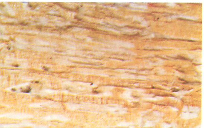
Figure 8 — White pockets of the advanced stage of decay of P. tomentosus in root wood.
