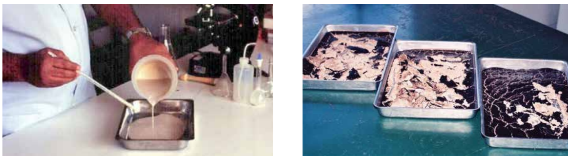
Figure 2. Baculovirus wettable powder preparation. Distribution in tray (left); Mixture of Baculovirus and kaolin clay, completely dry (right).
