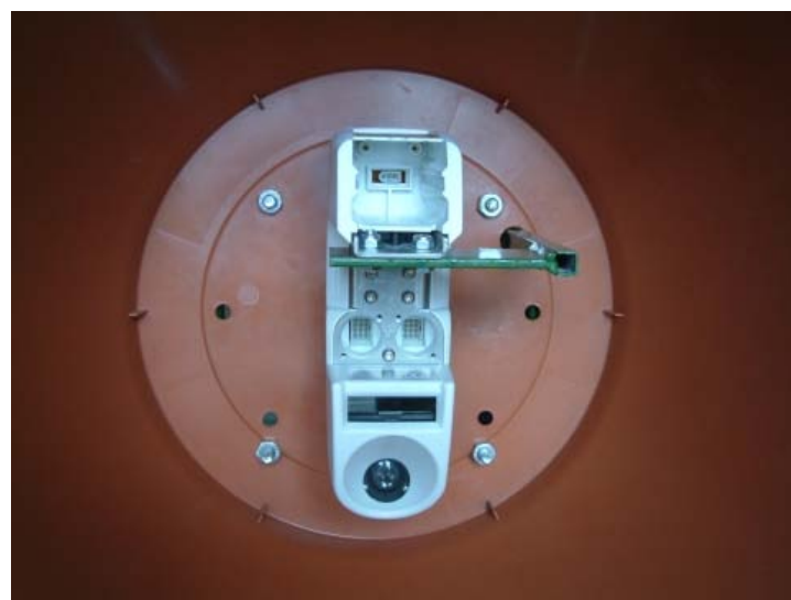
Figure 2. WeedSeeker sensor-sprayer shielded by plastic container (bottom view)
