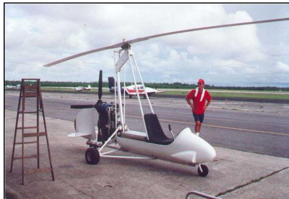
Autogir with FLI-MAP prototype
