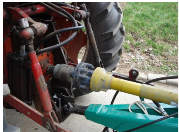
Fig.13. Machine connected to tractor's PTO. Mounting for registering the moment of resistance at PTO
