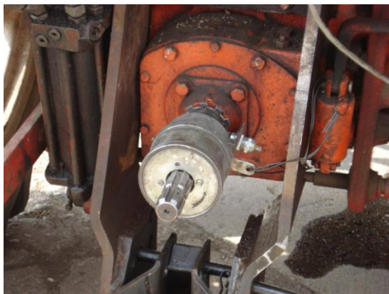
Fig.12. Dynamometer's mounting on tractor's PTO
