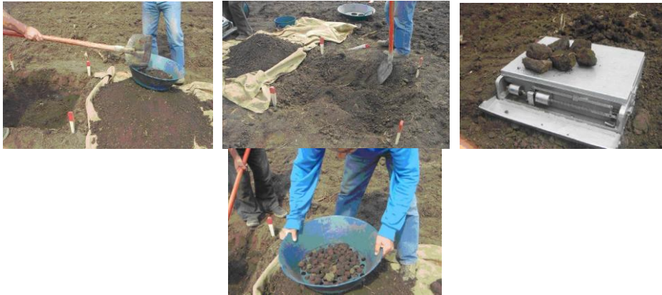
Determination of the soil's crumbling degree
