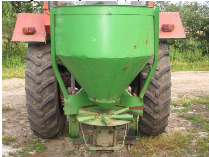
Fig. 6. The improve variant of the machine for administer solid chemicals.
