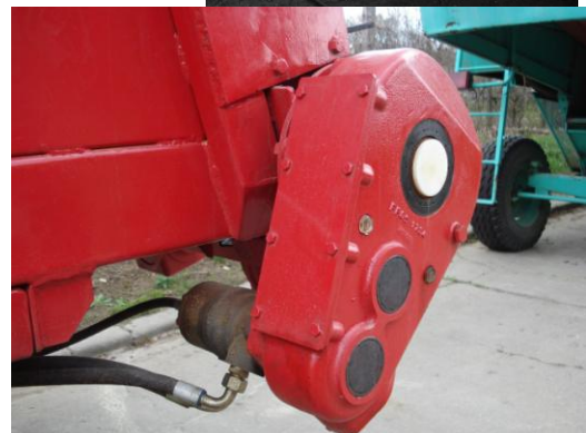
Fig.11. Conveyor's hydrostatic driving (a - discharge regulator; b- hydraulic engine + reductor )
