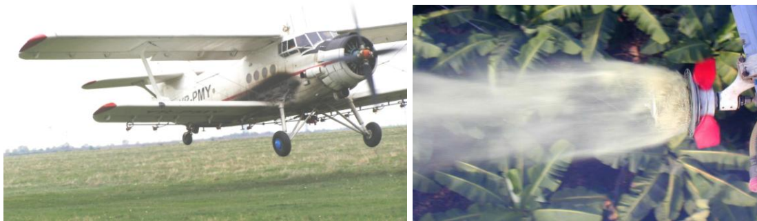
Figure 4. The plane AN-2 equipped with an spraying installation Micronair AU 4000, with 10 sprayers
