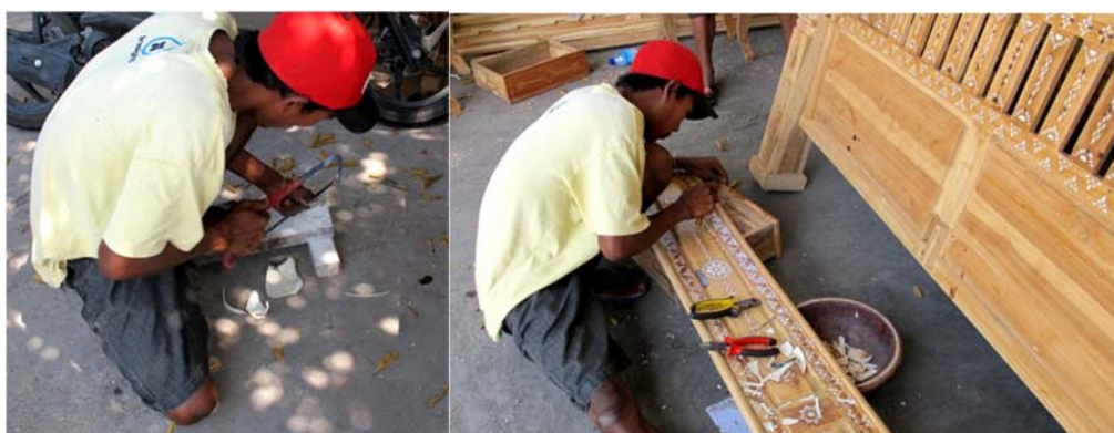
Figure 10: Small pieces of Nautilus shells are used to decorate wooden furniture. © WWF/TRAFFIC
