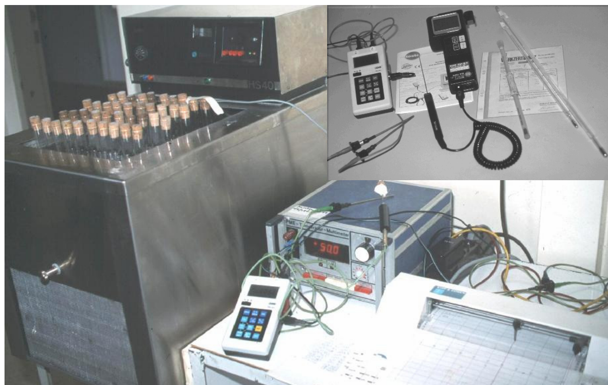
Figure 1. Water-bath with heated insect probes and temperature monitoring equipment
