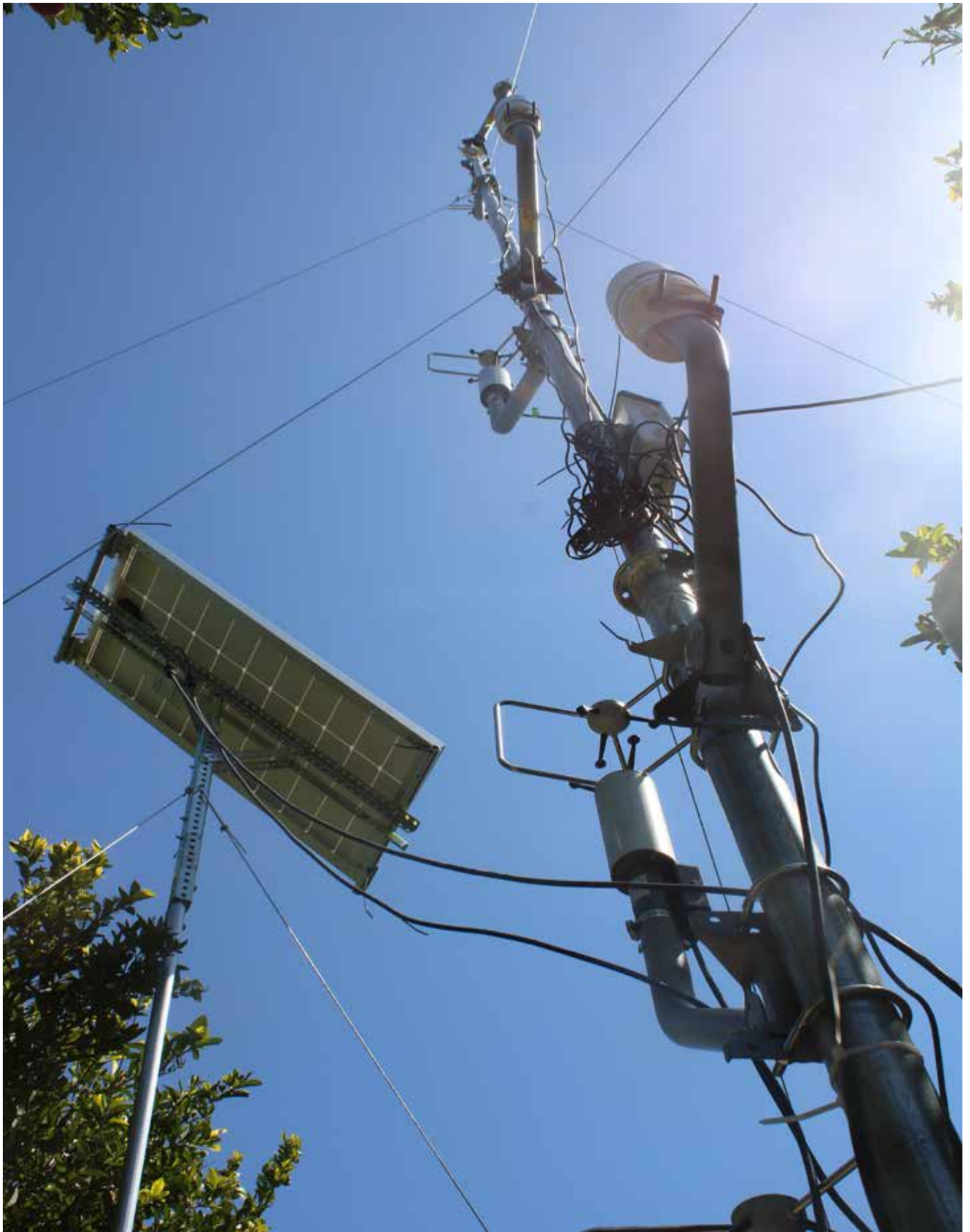
Figure 4. An auxiliary view showing parts of Met 1 weather station, including the uppermost two levels of weather instruments and a solar panel that was used to maintain electric power for the weather station.
