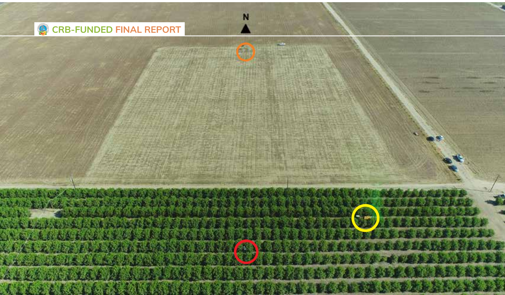
Figure 1. Oblique aerial view of the application area (orchard) and nearby sampling area (light colored area in open field). The sprayer (yellow circle) can be seen moving westward with drifting spray showing as a light green cloud at the rear. The locations of the weather stations are marked as red circle (Met 1) and orange circle (Met 2).
