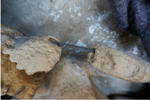
Figure 9: 'Rockbar' dowel used as armature for figure
