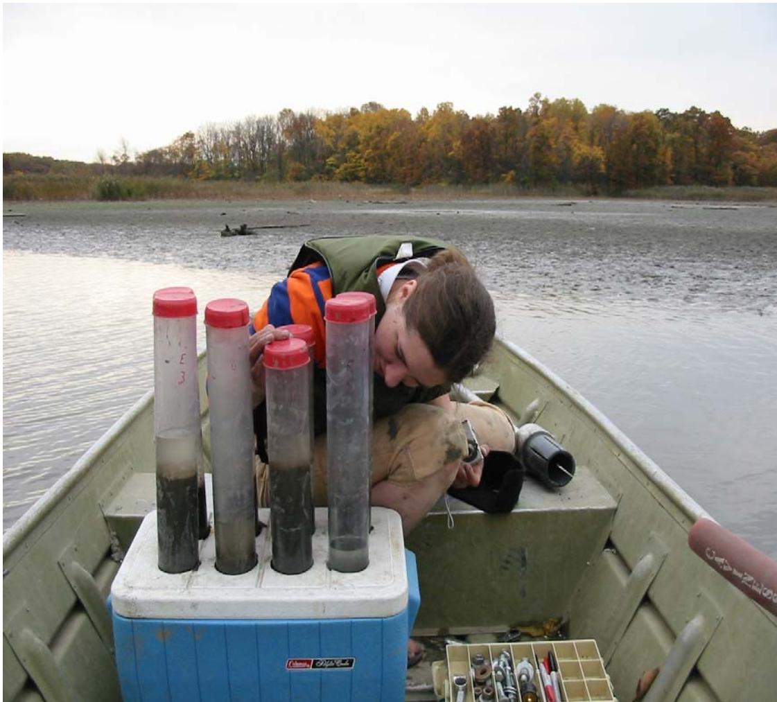
OSU researcher Alexandra Hakala collects sediment cores for pore water extraction from the estuary
