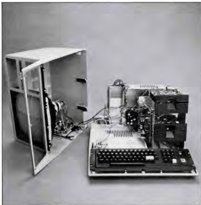
Photo 1. Model III with its computer case removed and lying on its side.
