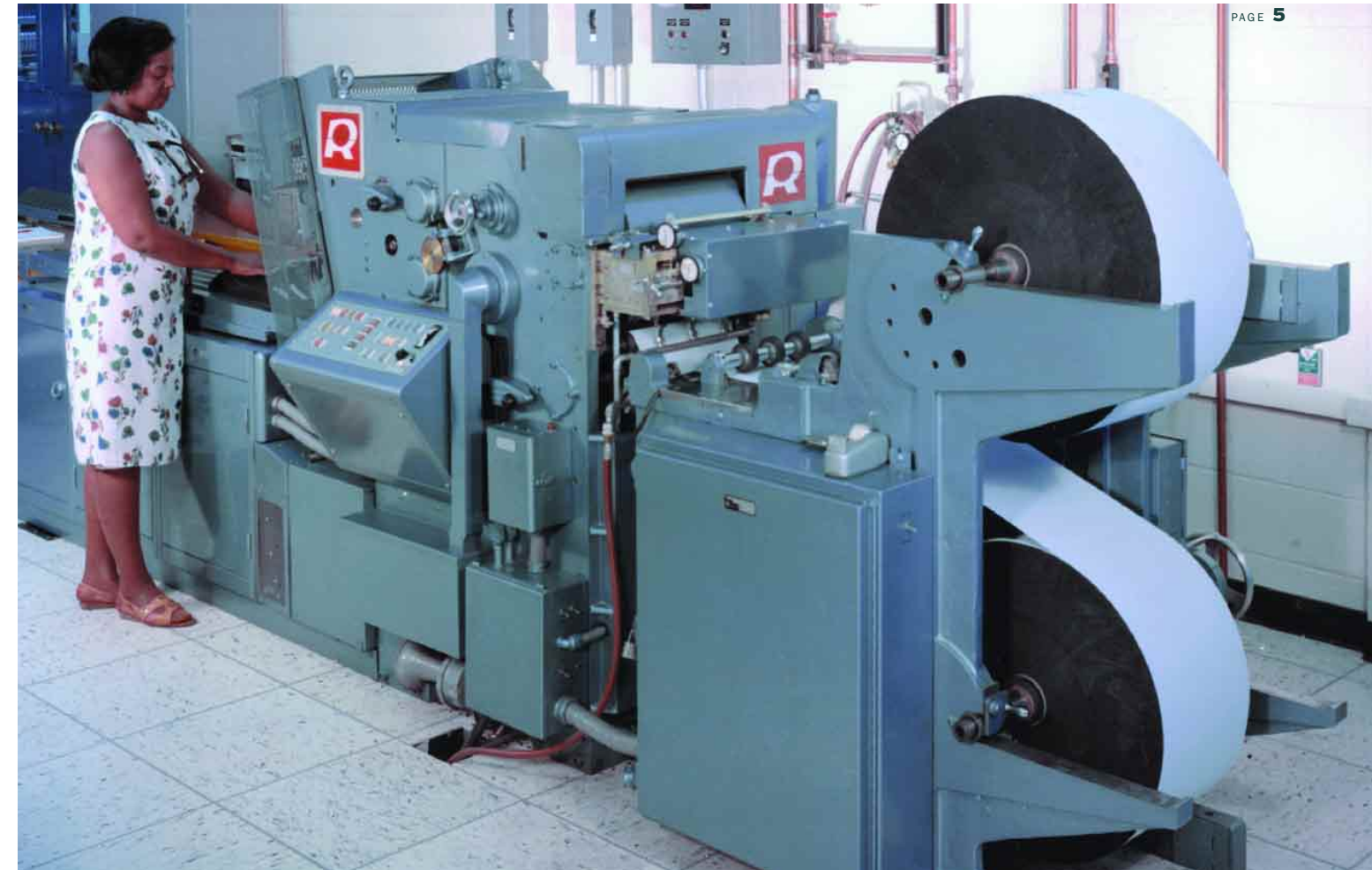
(above) Operator Mona Millings stands at the table where the separated output was delivered from the printer, and at the other end, the large rolls of paper used by the machine. Paper from the rolls could be spliced head to tail so there was no ordinary need for rethreading through the press. A roll lasted about 45 minutes and a special dolly was needed to move the rolls, since at over 200 pounds, they were far too heavy to be moved by hand.
