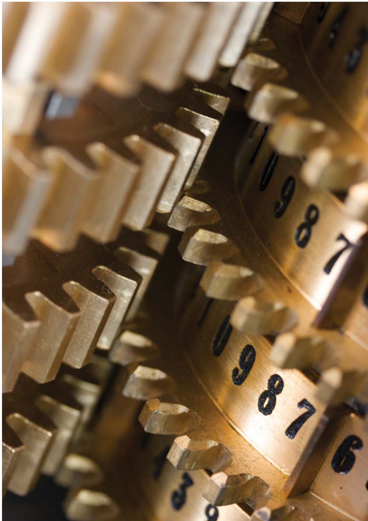
Figure wheels engaged with adjacent sector wheels during addition.
