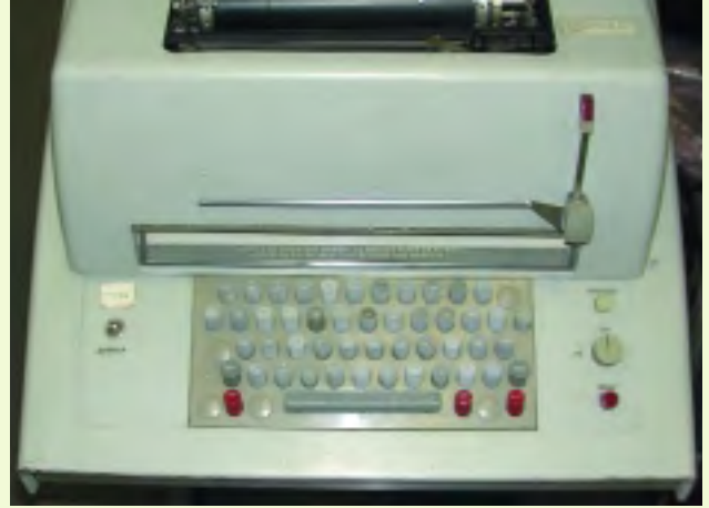
Console teletype. Through the mid-1970s, most mainframe computer systems used hardcopy terminal as consoles to aid in resource accounting, operator tasks, and general system debugging. The Sigma 5 was unusual in that it employed a TTY utilizing EBCDIC rather than the more common ASCII character encoding.
