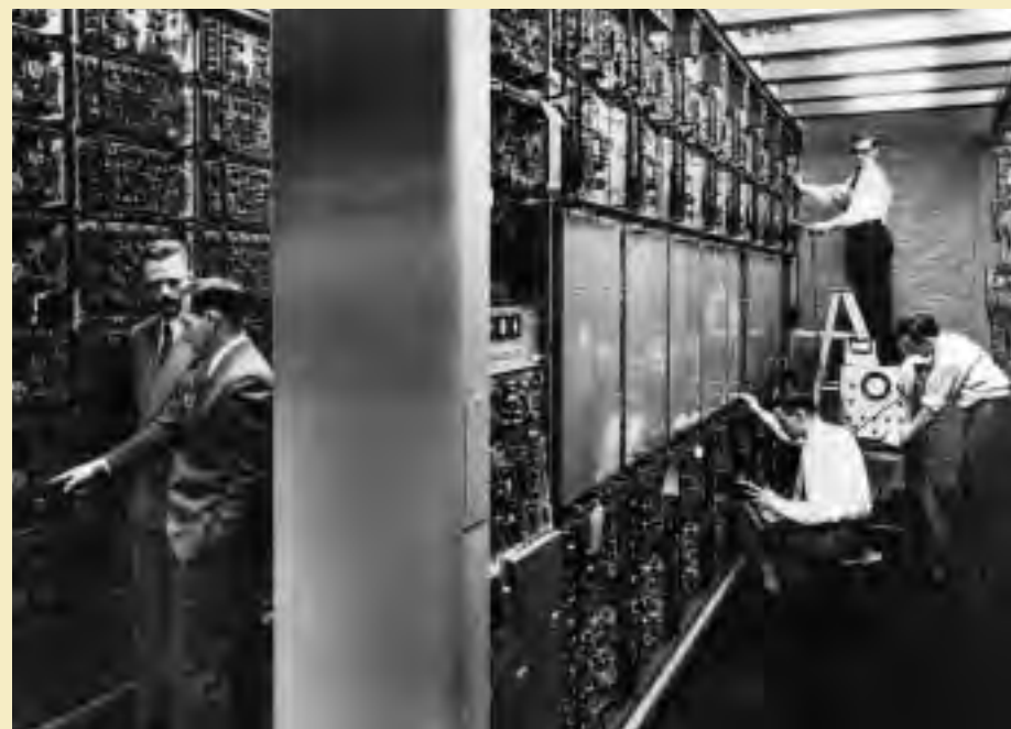
The internal workings of Whirlwind. Here, the machine's size dwarfs three technicians (John A. O'Brien, Charles L. Cordeiro, and Norman H. Dagger) working on the Electrostatic Storage Rack. At left, Jay Forrester and Norman H. Taylor inspect the Arithmetic Element Rack, 1952.
