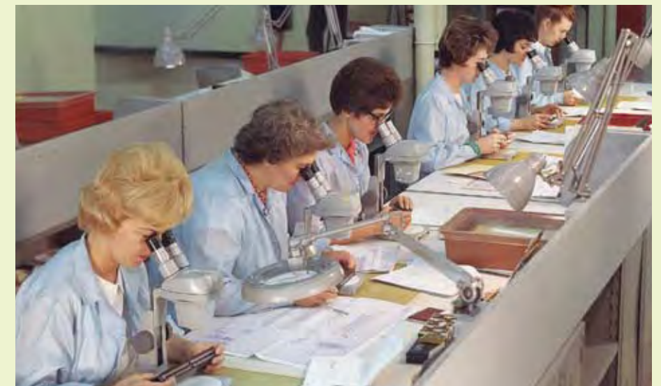
Assemblers at Raytheon testing and building AGC modules
