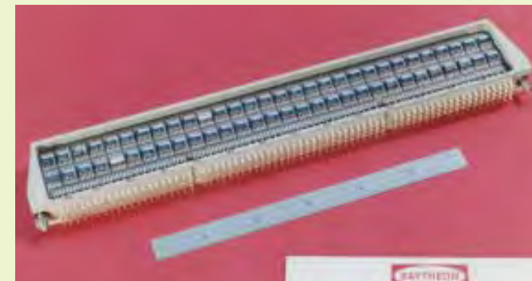
The module in the collection has been used only on Earth. The Museum's prototype computer ran at Draper Labs and was used to test the routines for in-flight machines. However, in space, all of the components had to be completely "potted" to insure that all the parts would stay firmly in place and remain uncontaminated.
