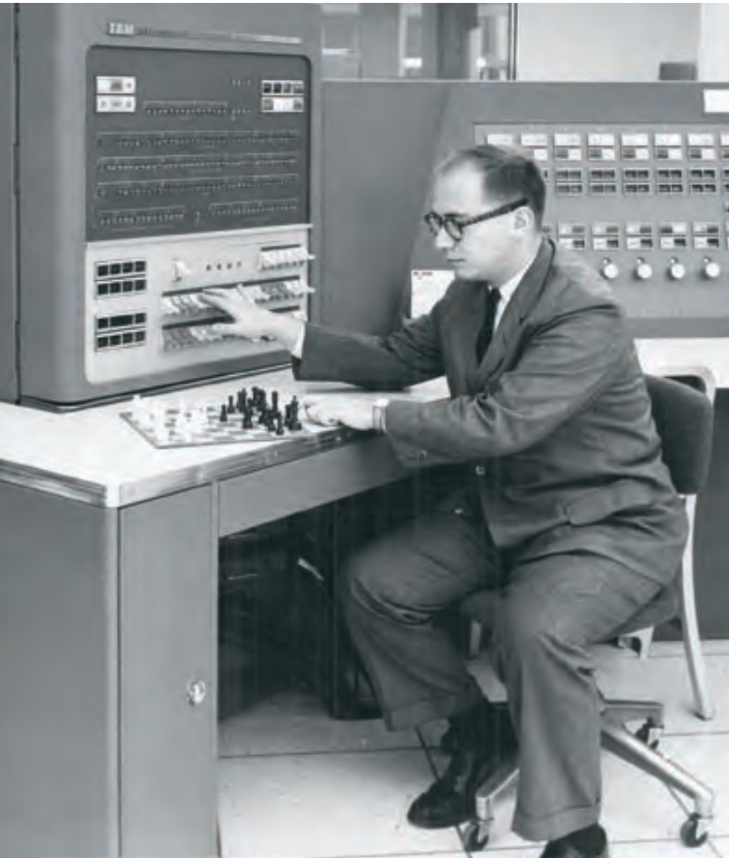
IBM programmer Alex Bernstein wrote a chess program for the IBM 704 mainframe computer in 1958. Bernstein told the computer what move to make by flipping the switches on the front panel. Courtesy of the IBM Archives, CHM# L02645391
