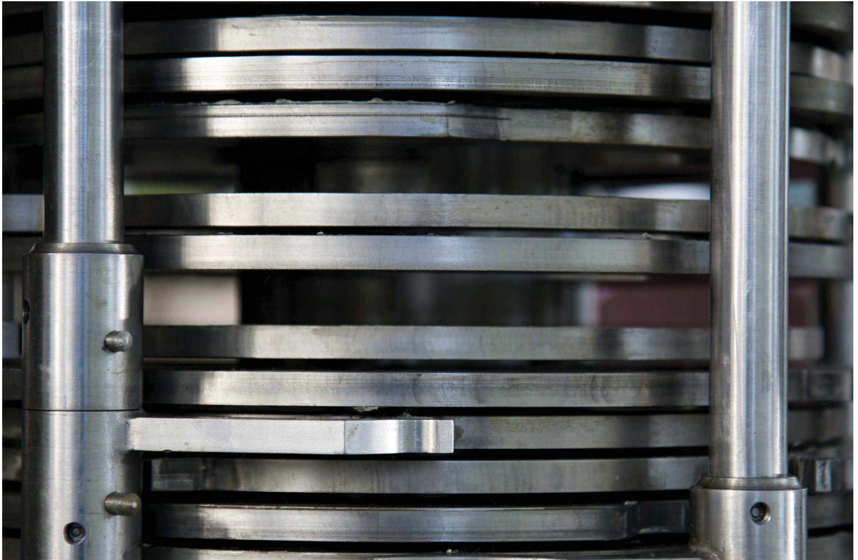
The subtle profiles of these cams encode the Engine's microprogram.
