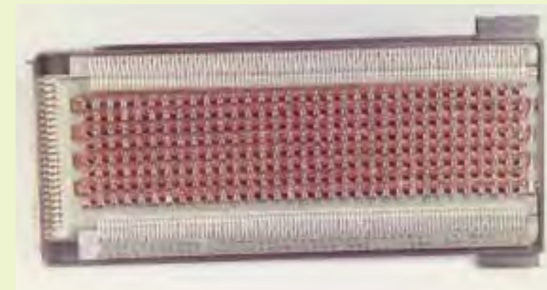
The read-only memory of the computer consisted of six rope memory modules, each containing 6,000 words of memory. This unique type of core memory treated each core as a transformer within a matrix of discrete "rope-like" wires and depended on the patterns set at the time of manufacture. Wires running through the core stored a "1," and those bypassing the core represented a "0." It had five times the density and was far more reliable than the coincident current core memory used for erasable storage in the computer. Being unalterable, it also provided a greater incentive for error-free software development.
