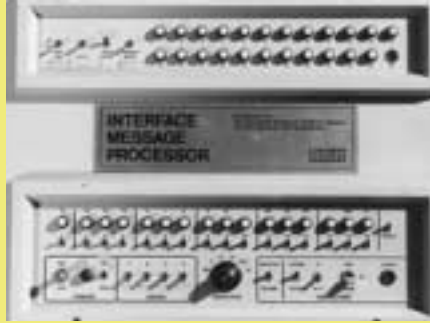
The IMP (Interface Message Processor), X105.82, Gift of Bolt Beranek and Newman, Inc.
