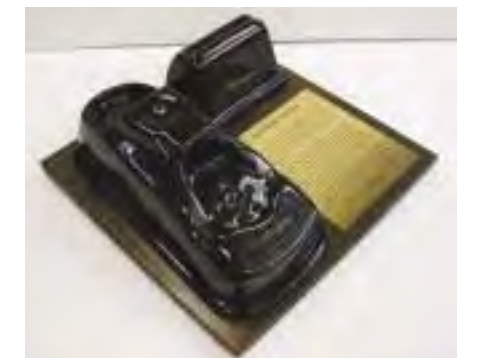
An original Carterfone, which sparked a debate that eventually led to the FCC's landmark "Carterphone decision," allowing third-party companies to manufacture and connect equipment to the public-switched telephone network (PSTN).
