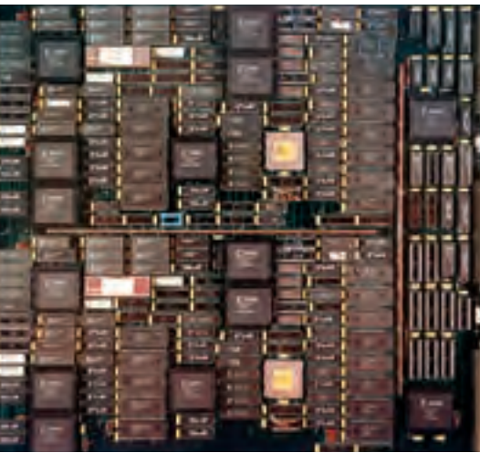
Deep Thought I circuit board, 1988 ca., 102645419, Gift of Feng-Hsiung Hsu. Carnegie Mellon University students Murray Campbell, Feng-Hsiung Hsu, Thomas Anantharaman, Mike Browne and Andreas Nowatzyk developed custom chess machine Deep Thought I in 1988.
