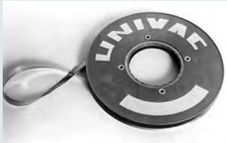
(above and right) With its "UNISERVO" tape drives, the UNIVAC was probably the first commercial machine to use magnetic tape as a storage medium. Customers initially resisted this technology since they could no longer "see" their data as they could with punch cards. IBM salesmen played up this fear, "hinting" that the UNIVAC, if it went out of control, could project shards of metal tape, potentially injuring or even killing customers.
