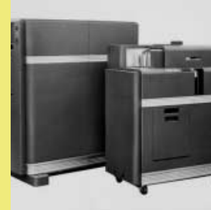
Museum volunteer and donor Robert Garner acquired and donated a 1948 IBM 604—a punched card calculator whose speed performance was due to its implementation with electronics (vacuum tubes), rather than IBM's traditional relay technology.
