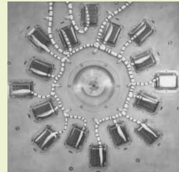
Librascope General Precision Model 30 (LGP-30) Drum Memory Unit (c. 1960), TCMHC photo #102621820 (P1631)
