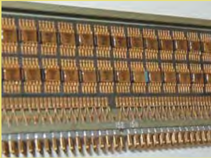
MIT Instrumentation Laboratory, Raytheon Company, Charles Stark Draper Laboratory Apollo Guidance Computer Prototype Processor-Logic-Interface-Memory modules (1962), X37.81B, Gift of Charles Stark Draper Laboratory
