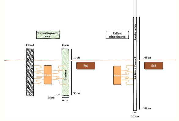
Sketch portraying the TroPeat ingrowth core and the EnRoot minirhizotron methodologies and their primary components. The medium used for the ingrowth core is homogenised peat from layers below the root mat.
