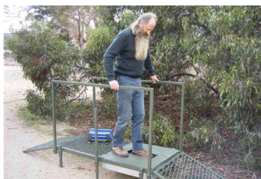
Figure A2.10 The 'Anakie Scrubber' footwear cleaning station consists of a metal ramp and disinfectant bath with an immersion plate for the cleaning of footwear prior entering uninfested areas (Photo: D Peters, Parks Victoria).
