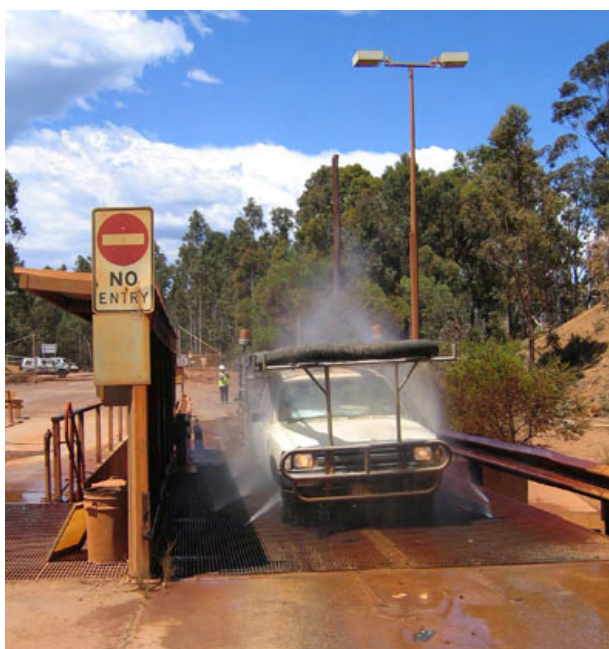
Figure A2.4 The automatic wash-down facility at the entrance to Alcoa's Huntly bauxite mine in the south-west of Western Australia, designed to remove soil from trucks and light vehicles entering the mine, thus minimising the probability of introducing Phytophthora cinnamomi to the predominantly disease-free site (Photo: E O'Gara).
