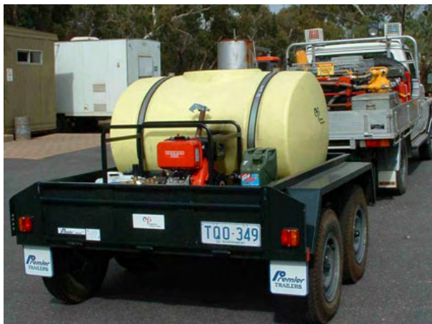
Figure A2.6 A portable wash-down unit. This type of system is used widely in South Australia and Western Australia to wash vehicles and equipment during general field and fire-fighting operations (Photo: R. Velzeboer, Department for Environment and Heritage in South Australia).
