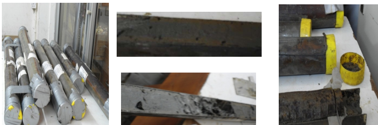
Figure 3.1. Photographs of the GCs during detailed sampling, with on the left, unsliced cores, in the middle, sliced cores and on the right, the detailed sampling resolution at 2cm.
