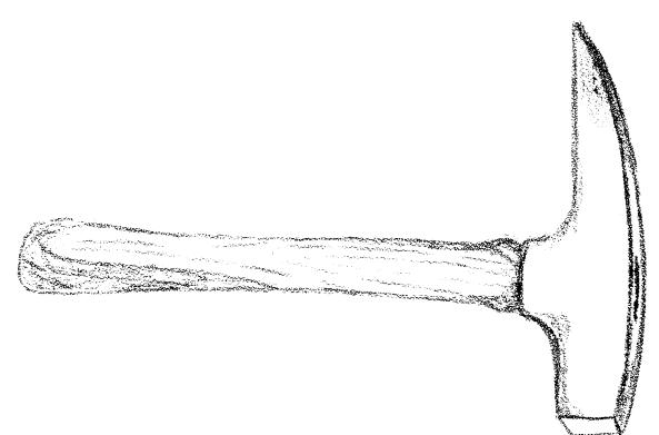
FIGURE 4. A geologist's pick or rock hammer, X1/2.
