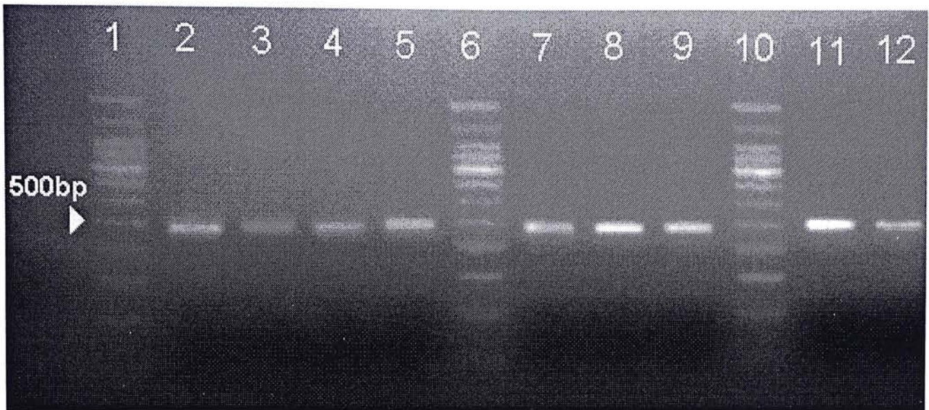
Figure 4.10. Agarose gel electrophoresis of the PCR products of the 5S rRNA spacer region. Lane 1, 6 and 10 are 100 base pair marker. Lane 2 is Stemona tuberosa (Chan200401) from the South China Institute of Botany. Lane 3 and 4 are Stemona tuberosa (ICM 20042541) from Yunnan. Lane 5 is Stemona tuberosa (Hu & But 23960) cultivated in Herb Garden of the Chinese University of Hong Kong. Lanes 7 to 9 are Stemona tuberosa (Woo 23973) from Guang Xi. Lanes 11 is Stemona parviflora (Ma 9066). Lane 12 is Stemona parviflora (Hu and But 24034).
