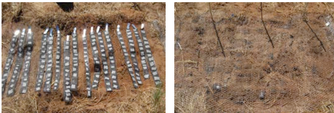
Figure 4.3. The flywire strips lightly buried in the field. (Left) and covered with chicken wire (Right).
