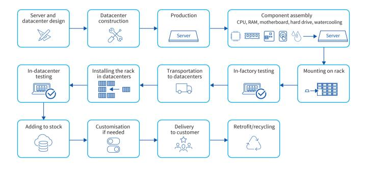
OVHcloud has two dedicated production sites – in France and in Canada – for assembling different hardware components into servers. Once the various components have been assembled, they are transported to the datacenter and customised as necessary prior to delivery to the customer. Since OVHcloud manufactures its servers in-house, it is not dependent on a third-party manufacturer, which reduces the risk of supply chain disruption.
