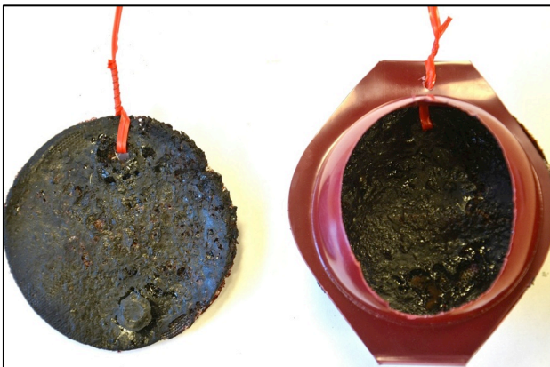
Figure 4. Two types of Attract and Kill stations (ATK) made of 3.5" woven polypropylene netting as a substrate, for raspberry concentrate, cider vinegar, yeast, gelatin, Super Absorbent Polymer (SAP) & 1% A.I. solution of insecticide.
