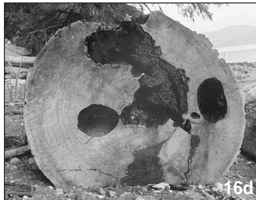
Figure 16a: Fruiting bodies of Neolentinus kauffmanii . Figures 16b, 16c, 16d: Characteristic brown pocket-rot symptoms of N. kauffmanii in Sitka spruce.
