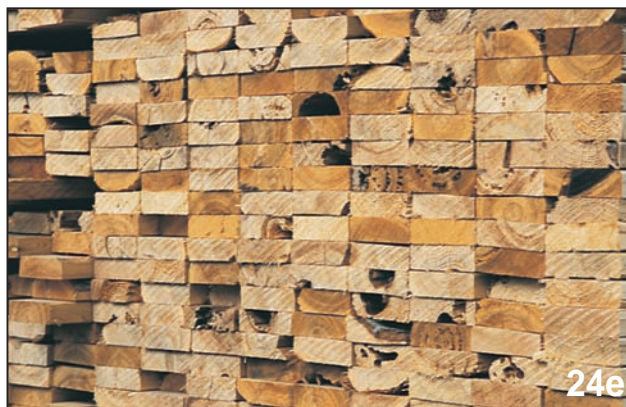
Figure 24a: Resupinate sporophore of Postia sericeomollis on western redcedar. Figures 24b, 24c, 24d: Brown cubical rot in western redcedar. Figure 24e: Brown cubical rot in cedar lumber.
