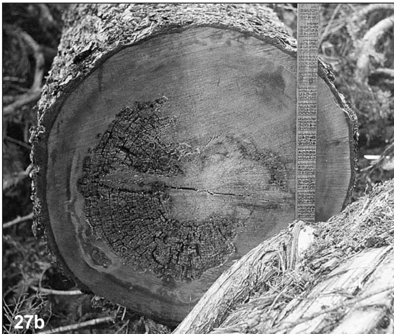
Figure 27a: Fruiting bodies of Veluticeps fimbriata on a fallen western hemlock log. Figure 27b: Advanced decay of western hemlock caused by V. fimbriata .
