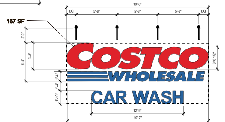
20 WALL SIGN FRONT SIDE SCALE: 1/4" = 1'-0"
