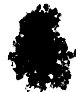
Figure 3. A fully hydrated aggregate consisting of 2-0.2 \mu\text{m} kaolinite clay particles and polyacrylamide (PAM), an organic flocculant, suspended in an aqueous solution of 0.01M \text{CaCl}_2 . (The kaolinite is the Clay Minerals Society source clay KGa-1. Clay content is 10 mg/mL. PAM content is 0.005 mg/mL.).
