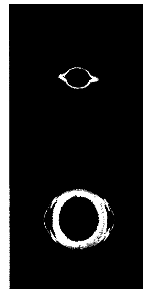
Figure 2. SAXS and WAXD Patterns. Strain=140%
