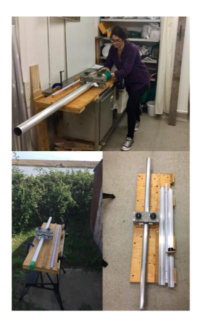
**Figure 8.** Fully assembled core slicer made at UCL Geography laboratory to slice 120cm aluminium cores: a) pre-cutting cores in lab; b) core processing in the field; c) whole and cut core in slicer
