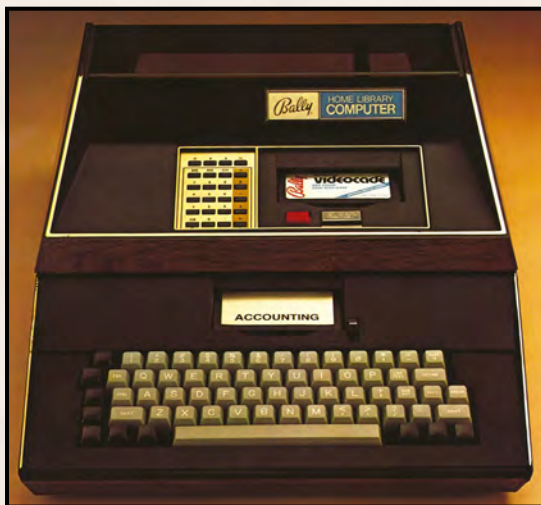
» [Fig. 10] DNA developed this hybrid game console and computer system in 1976, released in 1977. It was later renamed the Bally Professional Arcade and then Astrocade.
