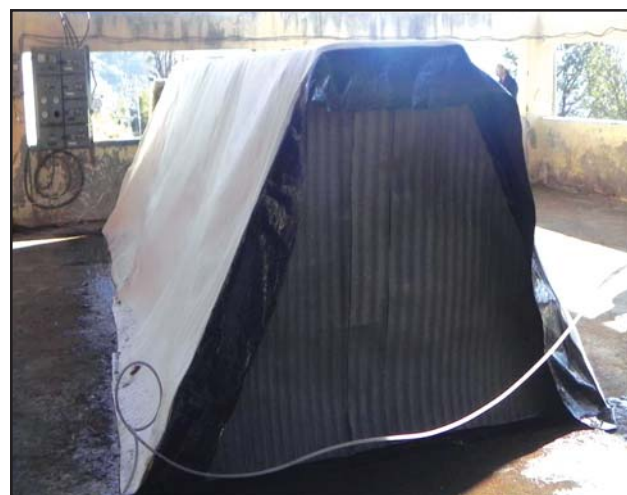
Fig. 2.23. Low cost pasteurization tunnel for button mushroom compost
