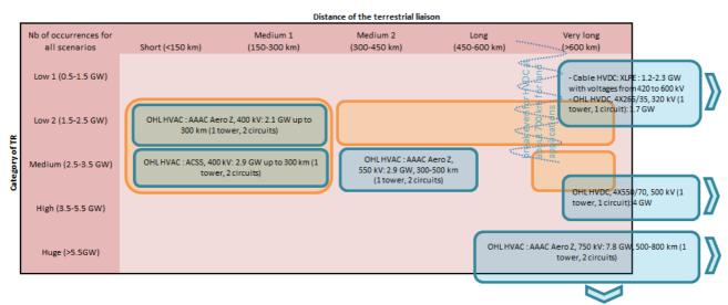
Figure 23: The technological options used in WP2 (in blue colour) compared to the needs (in orange colour) – terrestrial liaisons only
