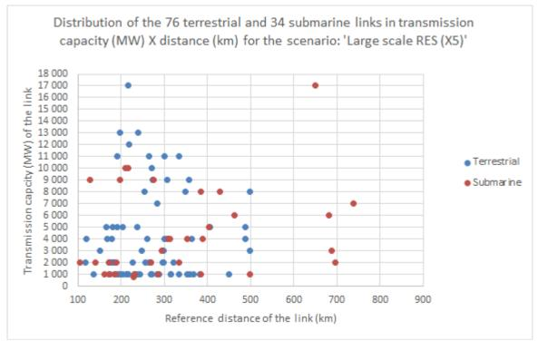
Figure 7: Distribution of the 110 links with non-zero TR for "Large scale RES" scenario
