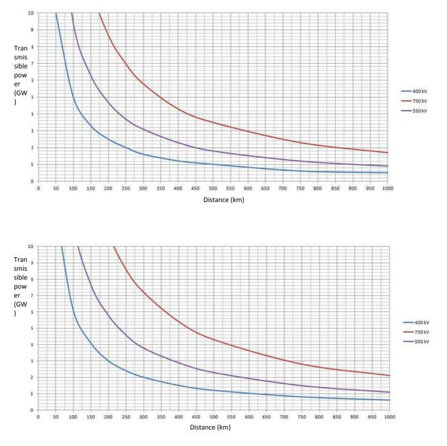
Figure 8 : Influence on maximum transmissible power over distance for different configurations of AC OHL (upper figure: two bundles per circuit; lower figure: four bundles per circuit)
