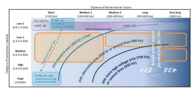
Figure 24: RD&D gap analysis: terrestrial needs (cells in orange colour) compared to available technology options (various grades of blue, from the more conventional to the less conventional)
