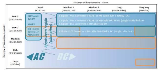
Figure 25: RD&D gap analysis: submarine needs (orange cells) compared to available technology options (blue cells)
