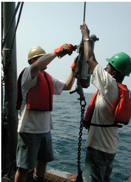
Figure 2.1-7 Preparing Niskin™ Bottle for Deployment
