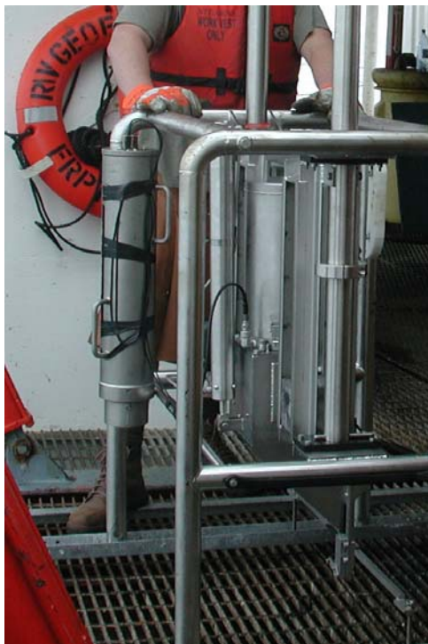
Figure 2.1-6 CTD Mounted on SPI Camera
