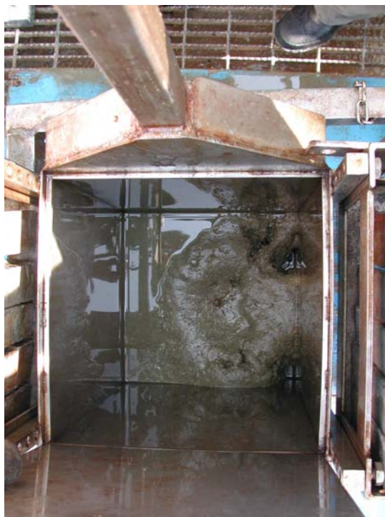
Figure 2.1-5 Undisturbed Sediment in Box Corer
