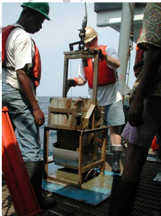
Figure 2.1-4 Box Corer on Deck After Sub-Sampling
