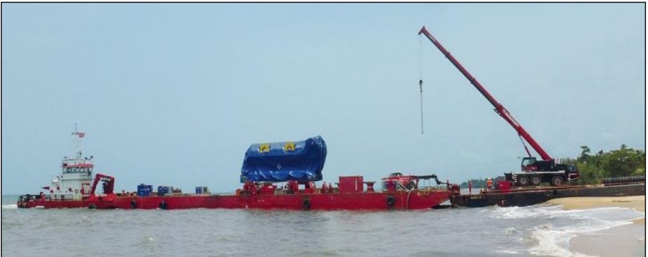
Figure 11: Typical beach landing site with barge offloading heavy equipment (source: Comarco)
