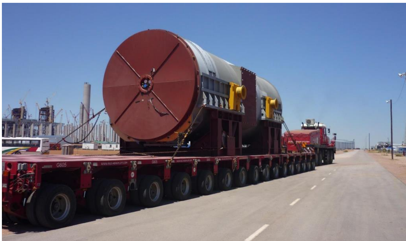
Figure 13: Heavy haulage truck with 16-axle hydraulic trailer transporting a 360-ton generator (source: ALE)
