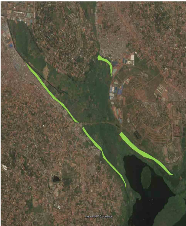
Figure A6.2 Proposed location of linear series of Cyperus papyrus wetland strip filters
