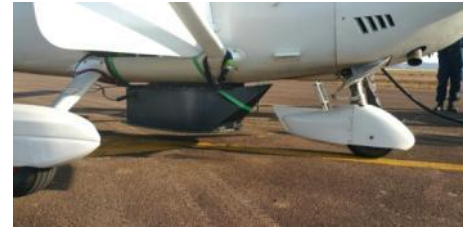
Figure 6. Aircraft and remote sensors container for airborne survey
