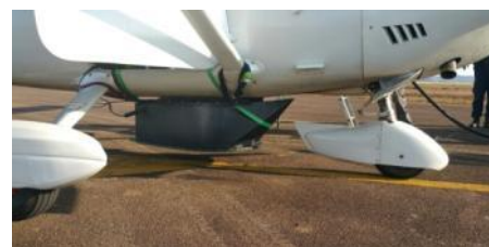
Figure 10. Aircraft and container of remote sensors for airborne survey
