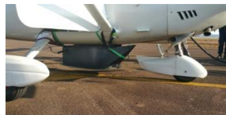
Figure 5. Aircraft and container of remote sensors for airborne survey
