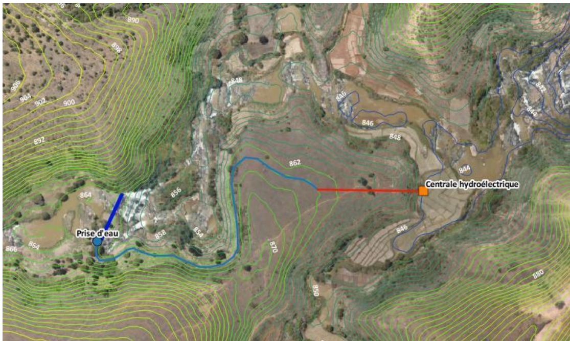
Figure 12. Proposed scheme layout for AD313 site (see also annex Erreur ! Source du renvoi introuvable.)
