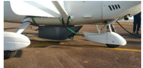
Figure 5. Aircraft and container of remote sensors for airborne survey
