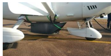
Figure 5. Aircraft and container of remote sensors for airborne survey
