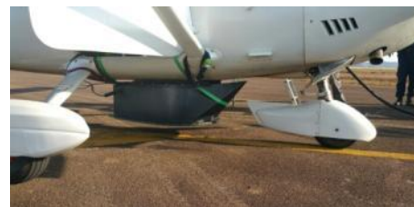
Figure 5. Aircraft and remote sensors container for airborne survey
