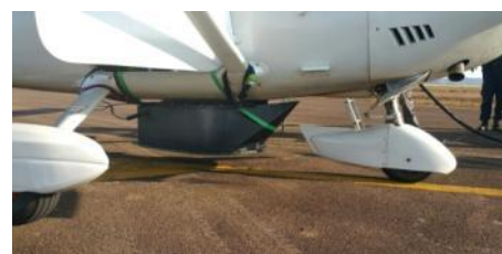
Figure 6. Aircraft and container of remote sensors for airborne survey
