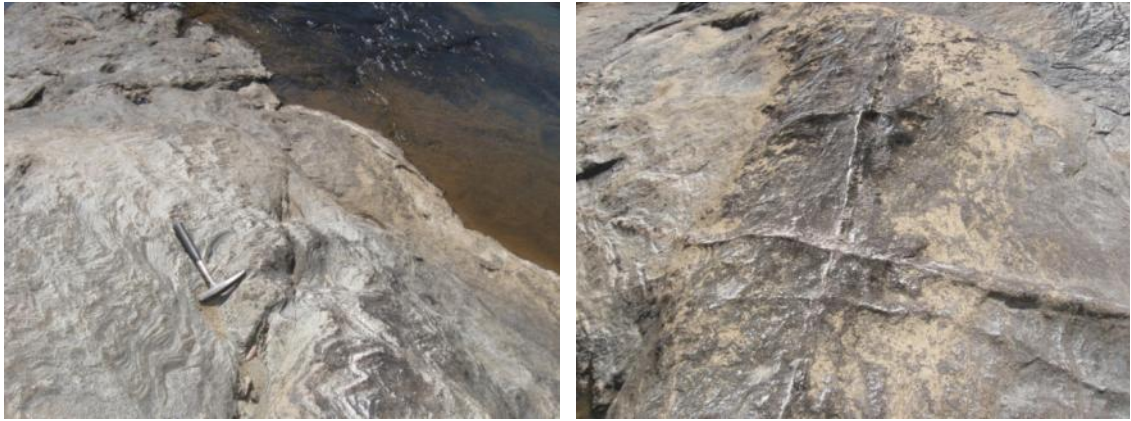
Figure 9. Medium to fine grain, granitoid like, biotite migmatite with quartz and feldspar
