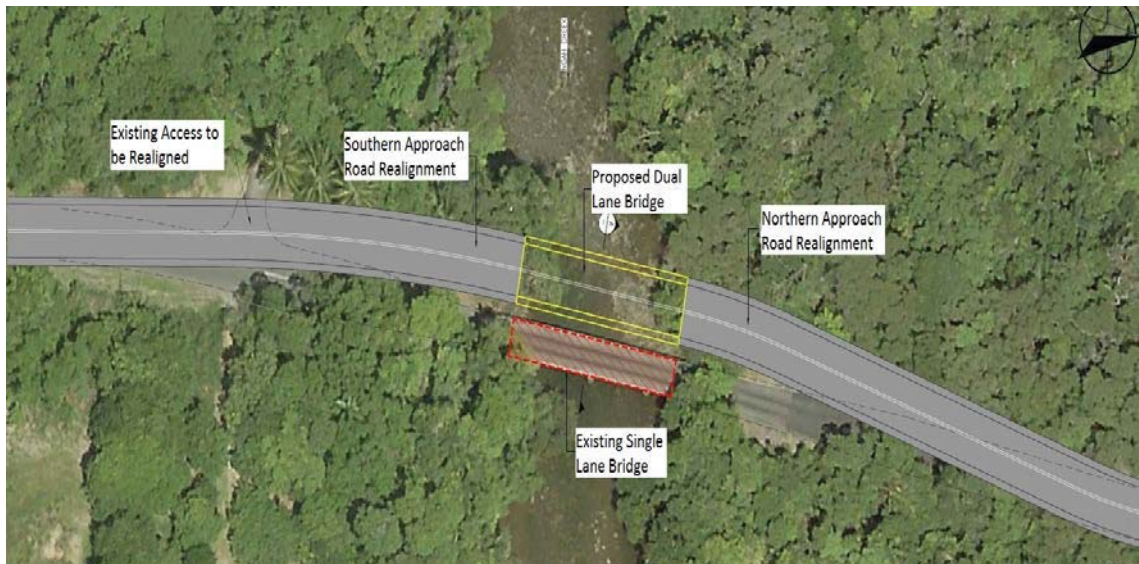
Figure 1 Proposed Bridge Replacement
