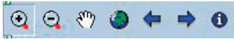
The MapViewer template's toolbar already contains tools and commands for navigating the map (Zoom In, Zoom Out, Pan) and for identifying features in the map.
