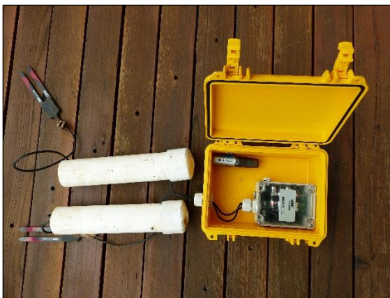
Figure 15. Refurbished soil moisture logger in Pelican box (left) and placement of box at 10 cm from surface (right).
