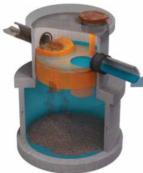
Figure 3 – HumeCeptor® system operation during design flow condition
