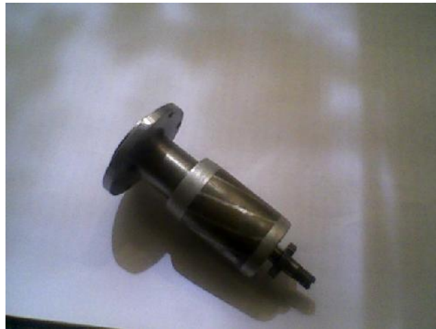
Photo. 2. Flexible squirrel cage rotor.
