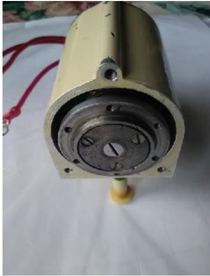
Photo. 1. High-speed three-phase asynchronous electric motor with a cantilever squirrel cage rotor
