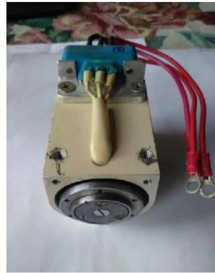
Photo. 1. High-speed three-phase asynchronous electric motor with a cantilever squirrel cage rotor
