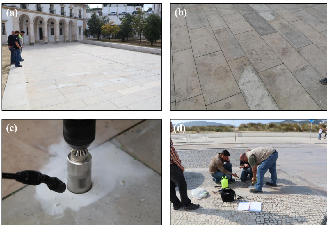
Figure III-3. Sampling process of the building stone located at the floor pavements next to the Mosteiro da Batalha building (a), (b), (c) and in the waterfront of São Martinho do Porto village (d). ©Luís Lopes
