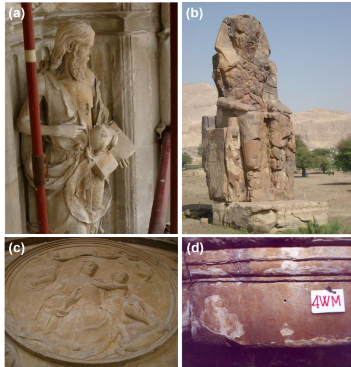
Figure I-22. Examples of weathering in pieces of art made of limestone and marble. Patina formations (a, b and c) and a hardened crust formed after a past treatment (d), responsible for the detachment of a thin stone layer (adapted from Rodrigues, 2006).
