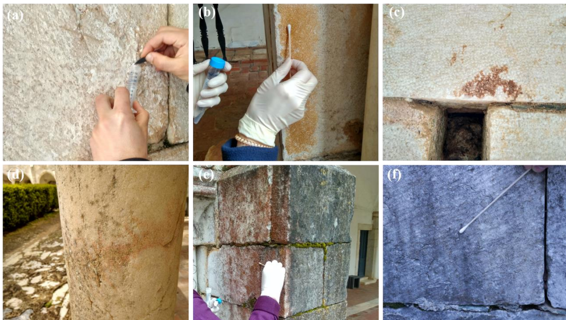
Figure V-5. Areas selected for the methodology approach. Areas CM1 and CM2 correspond to white and yellow patinas (a, b), areas CM3 and CM4 correspond to reddish stains and fissures (c, d), areas CM5 and CM6 correspond to formation of red and dark biofilms (e, f).
