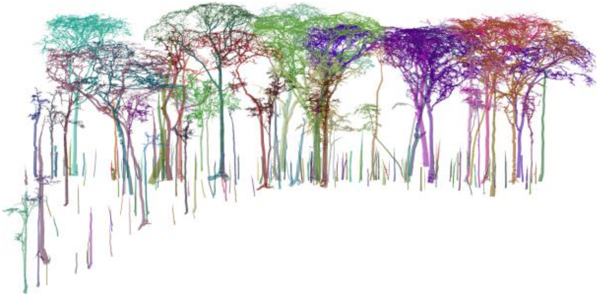
Figure 11 Individual tree point clouds extracted from the AfriSCAT plot (top); the same trees reconstructed as cylinder models (bottom). Trees which are shown trunk-only are those with 10\text{cm} \leq \text{dbh} < 20\text{cm} .
