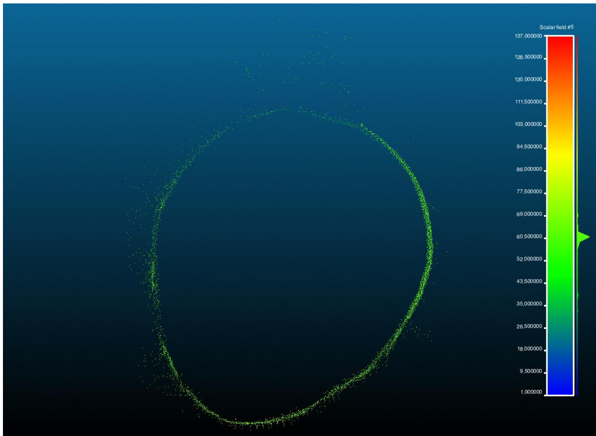
Figure 9 Example illustrating the accuracy of co-registration of the merged TLS point cloud. Colours represent points from different scan locations within the point cloud.
