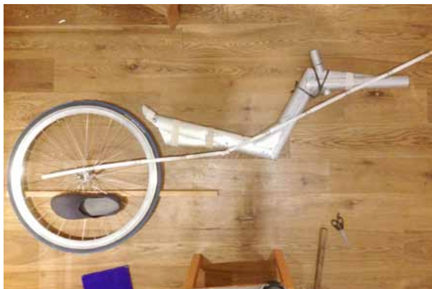
Model 2 – checking the frame layout with prospective chain line (folding rule).
