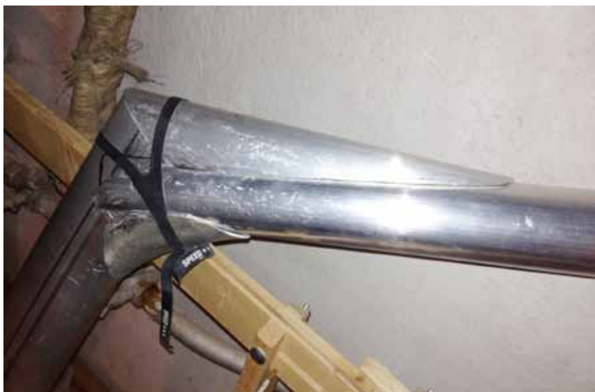
Model 2 – reinforced front part of the Z-frame.
