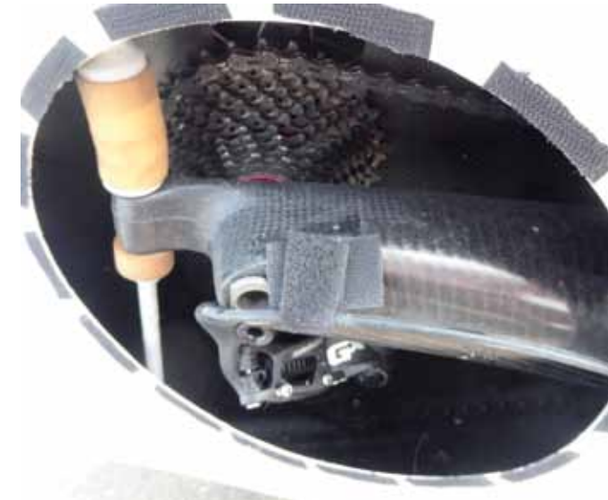
Carbon swingarm with pull rod and elastomers.
