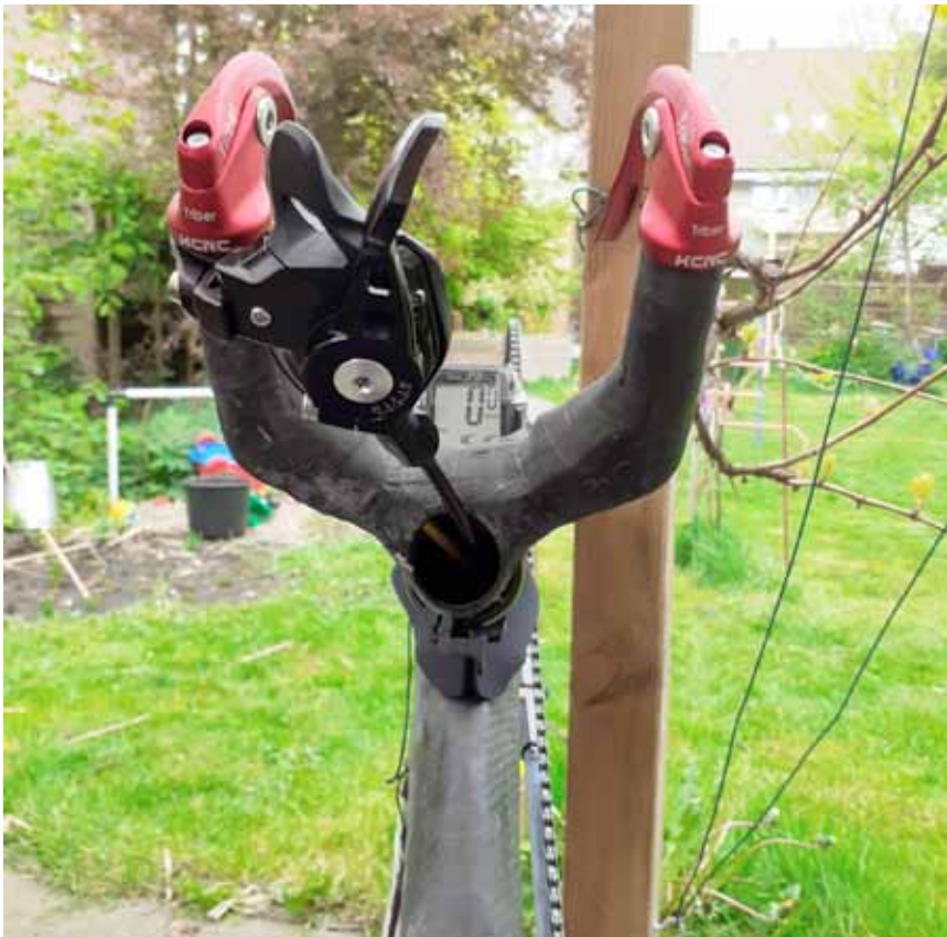
Cockpit of model 5 with integrated speedometer.
