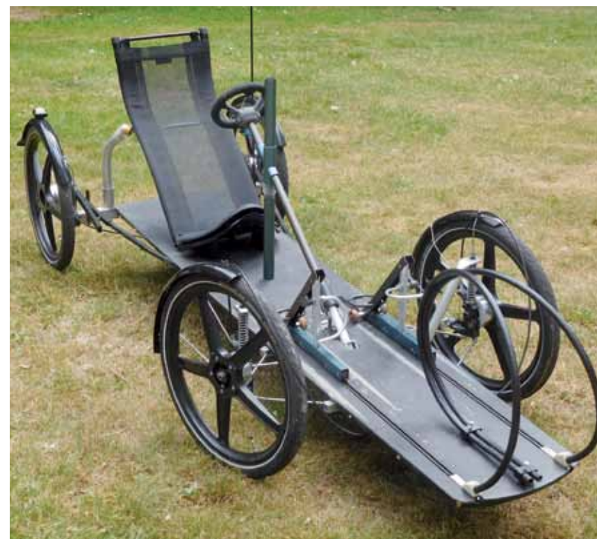
Each pedal engages onto its own belt. This belt is wrapped around the free-wheel on the rear wheel axle.
