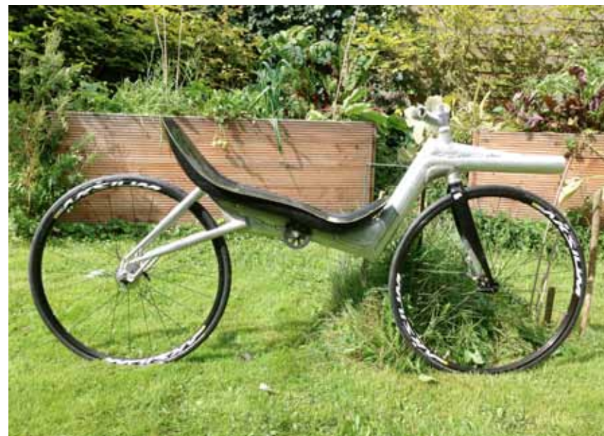
Model 2 – the naked frame, ready welded.
