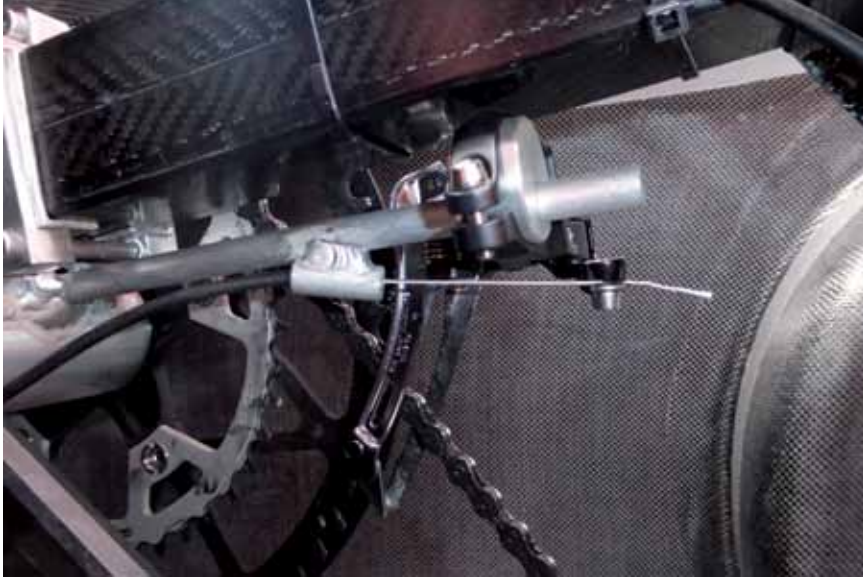
Crankset fitted under the nose pipe.
