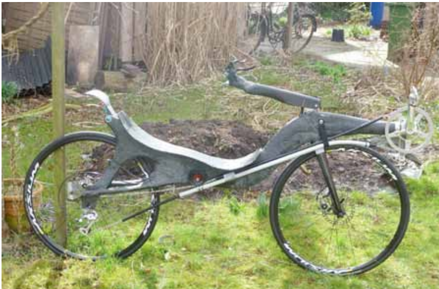
Model 3, my first real "self-construction" made from carbon.
