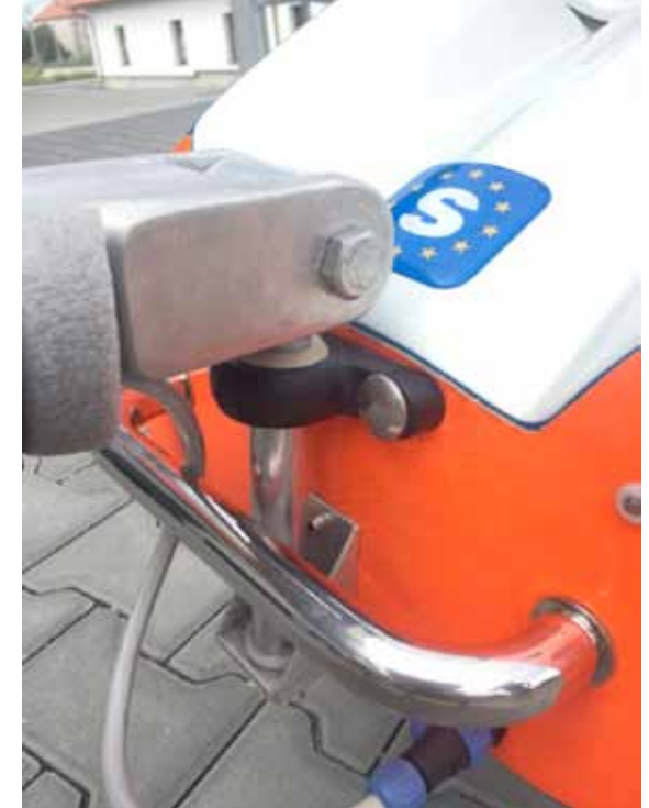
Very well thought out trailer attachment which caused Alve's visit to Azub at the end. Well, all parts need some testing and some of them fail sooner or later. This one did so later, but after some little improvement, we believe will work safely till the end of the journey.
