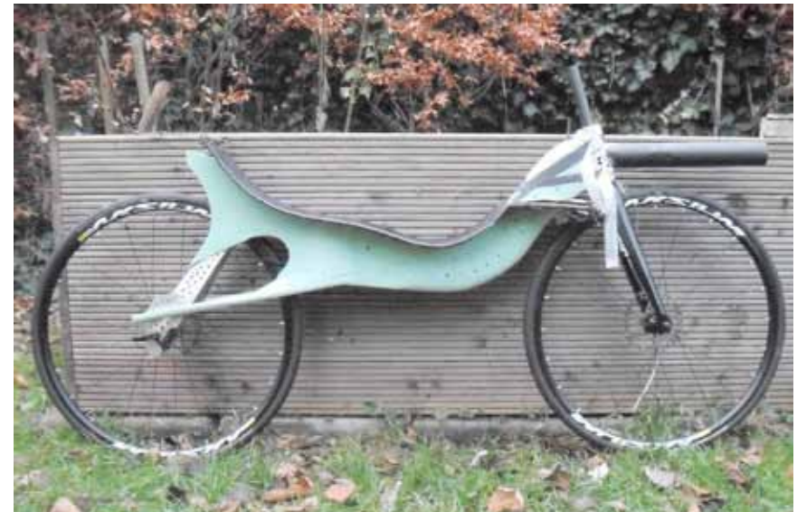
Model 3, PVC foam body and aluminum compounds.
