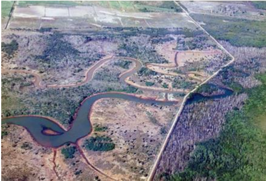
Figure 2.3.11: Mangrove dieback as a result of the bund wall and the release of sulphuric acid from acid sulphate soils in the 1980s (photo DEHP)
