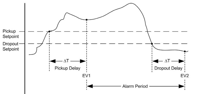
**EV1** An alarm is active. The power meter records the date, time, and value at EV1 when the pickup setpoint and time delay are satisfied. The power meter performs any tasks assigned to the event such as operation of a digital output, backlight flashing, and alarm symbol flashing.
