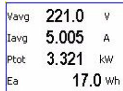
Full screen mode is enabled by default. You can modify full screen enable/disable information, auto scroll enable/disable, and auto scroll interval in HMI configuration.
