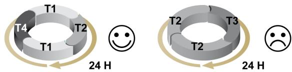
In the setup of a scheduler, you should define the tariff switching time and the target tariff rate from the switching time. In the application, when the set switching time reaches, the current tariff rate switches to the target rate automatically.
