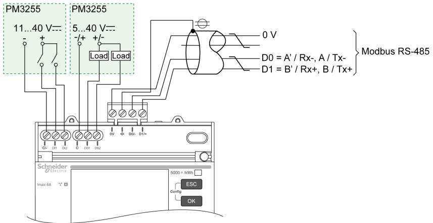
**NOTE:** The electrical wiring is explained in the table below.
