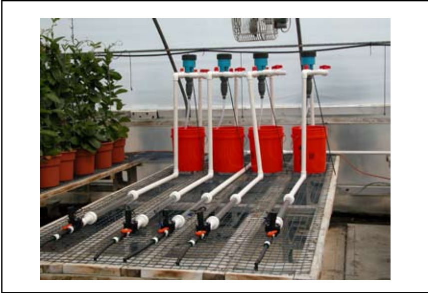
Figure 8. Experimental irrigation matrix for researching biofilm and algae in irrigation lines.
