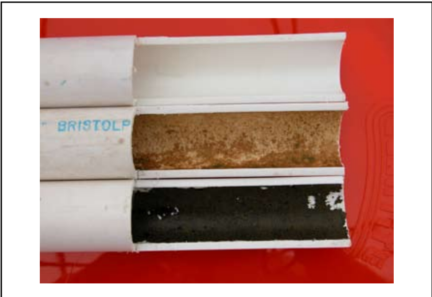
Figure 7. Longitudinally cut PVC mains; top section is new, middle section carries clear water, bottom section carries fertilizer. Note discolored biofilm layer in clear section and algae dominated layer in bottom section.
