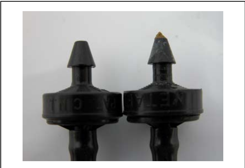
Figure 4. Algae and biofilm cause clogging of drip emitters. New emitter on left, clogged on right.
