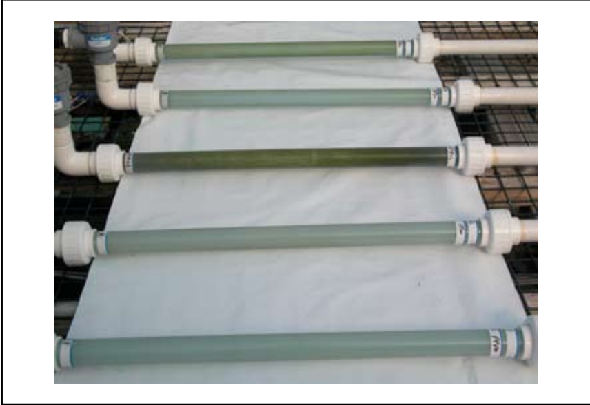
Figure 11. Clear sections of lines following continuous injection of Selectroicide with untreated control in center.
