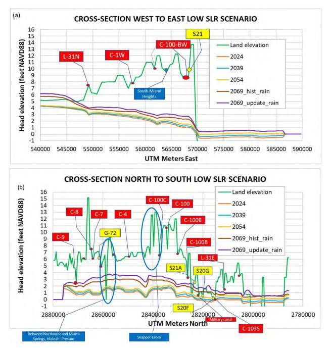
Figure 67. Cross-section for low SLR scenario and sensitivity runs (a) West to East and (b) North to South.
