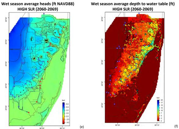
Figure 76. Left panel: Average wet season heads (ft NAVD88) for (a) Calibration run (1996-2010), (c) Low SLR run (2060-2069), (e) High SLR run (2060-2069). Right panel (b), (d), (f): Average wet season depth to water table (ft) for the same runs.
