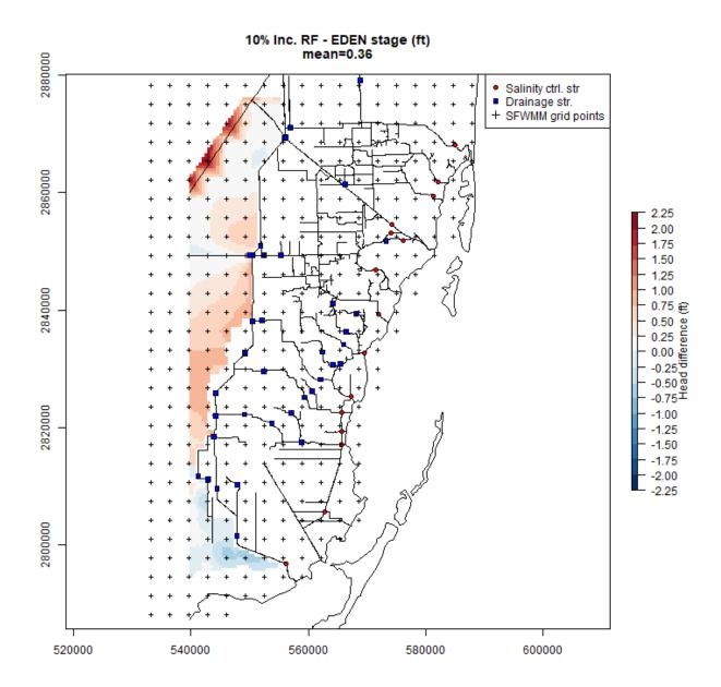
Figure 46. Differences between simulated stages in the 10% increased rainfall scenario (1965-2005) and the EDEN dataset (1996-2010). X and Y coordinates in meters, UTM17N, NAD83.
