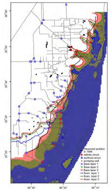
Difference in freshwater/saltwater interface HIGH SLR vs. CALIBRATION
