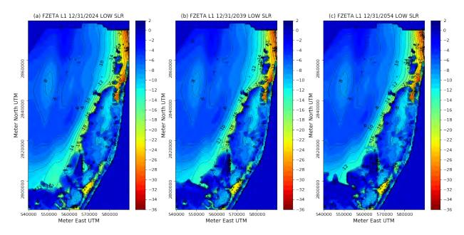
Figure 69. Zeta surfaces of layer 1 low SLR scenario for (a) 12/31/2024, (b) 12/31/2039, (c) 12/31/2054.
