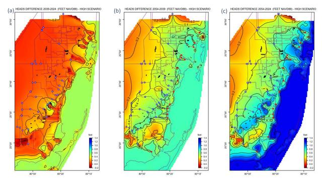
Figure 65. Simulated difference in heads for high SLR scenario between (a) 12/31/2039 and 12/31/2024, (b) 12/31/2054 and 12/31/2039 and (c) 12/31/2054 and 12/31/2024.
