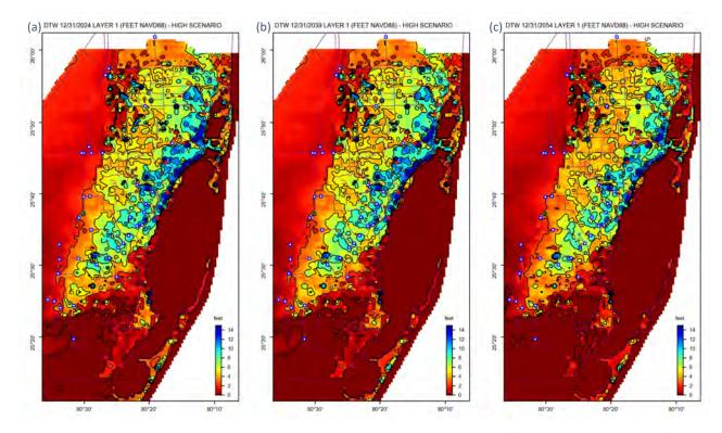
Figure 63. Simulated depth to water of High SLR scenario on (a) 12/31/2024, (b) 12/31/2039 and (c) 12/31/2054
