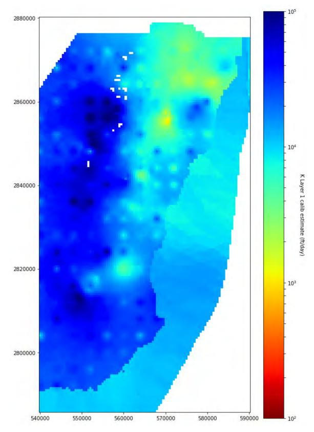
*Figure 12. Back-calculated calibrated hydraulic conductivity for layer 1, K\_cell.*
