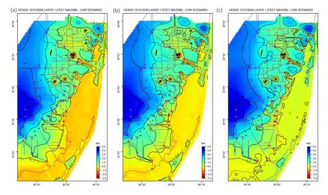
Figure 60 . Simulated heads of Low SLR scenario on (a) 12/31/2024, (b) 12/31/2039 and (c) 12/31/2054.
