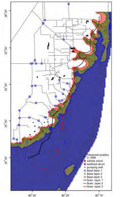
Difference in freshwater/saltwater interface (HIGH SLR + NO PUMPAGE) vs. HIGH SLR
