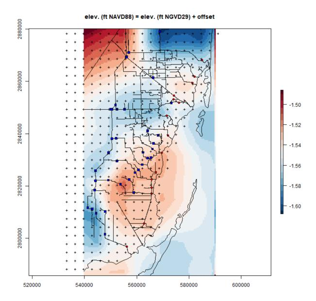
Figure 47. Datum shift offsets for the MODFLOW model domain (elevation in ft NAVD88 = elevation in ft NGVD29 + offset). X and Y coordinates in meters, UTM17N, NAD83.
