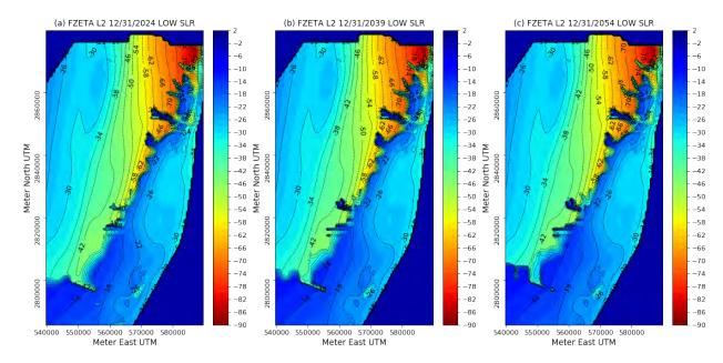
Figure 70. Zeta surfaces of layer 2 low SLR scenario for (a) 12/31/2024, (b) 12/31/2039, (c) 12/31/2054.
