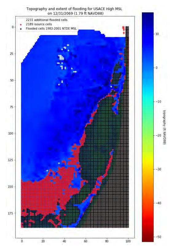
Figure 51. Topography and extent of flooding (cells with '+' black and white markers) for mean sea level on 2069 at Virginia Key for the USACE High SLR scenario (1.79 ft NAVD88). A total of 2231 additional model grid cells would be below MSL. X and Y coordinates in meters, UTM17N, NAD83.
