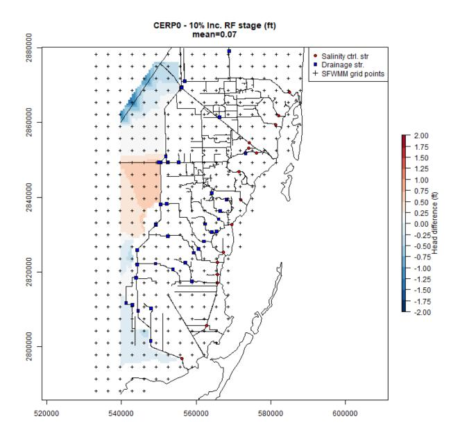
Figure 44. Differences in average simulated stages between the CERPO scenario and 10% increased rainfall scenario (1965-2005). X and Y coordinates in meters, UTM17N, NAD83.
