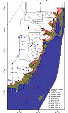
Difference in freshwater/saltwater interface (HIGH SLR + HIST RAIN/RET) vs. HIGH SLR
