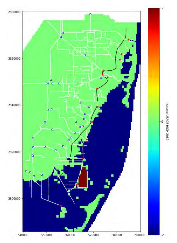
Figure 52. Freshwater/saltwater source (isource) based on the mean sea level on 2069 at Virginia Key for the USACE High SLR scenario (1.79 ft NAVD88). X and Y coordinates in meters, UTM17N, NAD83.
