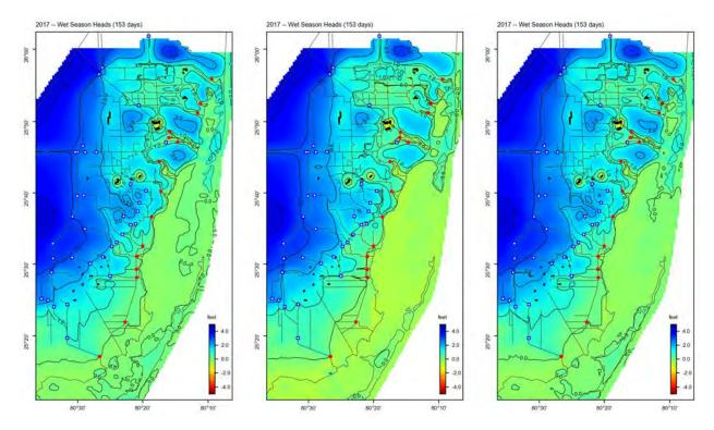
Figure 16. 2017 simulated average wet season heads in feet NAVD. Heads based on observed tide water level input (left), predicted tide without trend input (center), and predicted tide with added trend (right). Red dots are salinity control structures. White boxes with blue outlines are water supply/flood control structures.
