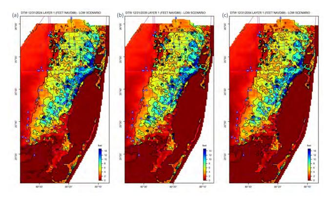
Figure 61. Simulated depth to water of Low SLR scenario on (a) 12/31/2024, (b) 12/31/2039 and (c) 12/31/2054.
