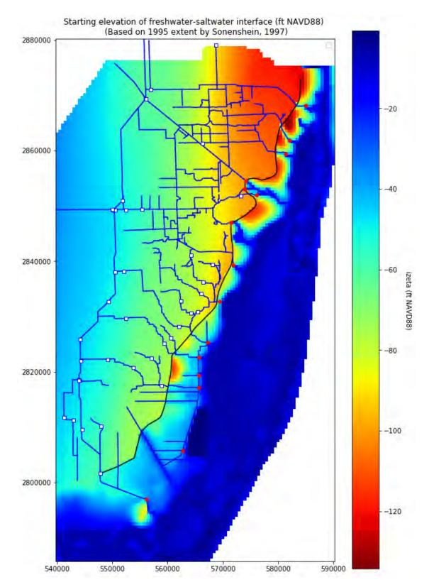
Figure 53. Starting elevation of the freshwater/saltwater interface in 1996. X and Y coordinates in meters, UTM17N, NAD83.
