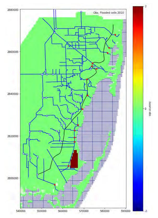
*Figure 86. Freshwater/saltwater source (isource) for the 1996-2010 calibration run. Cells marked with white '+' are below the 2010 historical mean sea level at Virginia Key and their isource value is (for the most part) equal to -2 (blue).*
