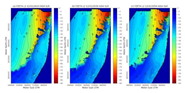
Figure 73. Zeta surfaces of layer 2 high SLR scenario for (a) 12/31/2024, (b) 12/31/2039, (c) 12/31/2054.
