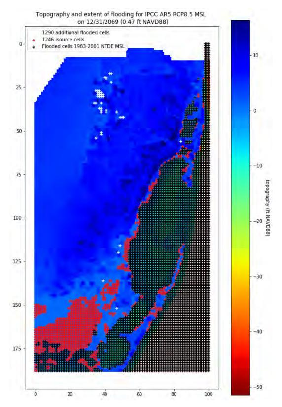
Figure 49. Topography and extent of flooding (cells with '+' black and white markers) for mean sea level on 2069 at Virginia Key for the IPCC AR5 RCP8.5 SLR scenario (0.47 ft NAVD88). A total of 1290 additional model grid cells would be below MSL compared to the cells flooded based on 1983-2001 NTDE MSL. X and Y coordinates in meters, UTM17N, NAD83.
