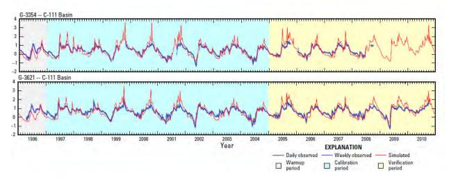
Figure 83. Observed and simulated water levels in the calibration/verification run for wells in the C-111 Basin. From Figure 5-5 Hughes and White (2016), with permission. Vertical units are ft NAVD88.
