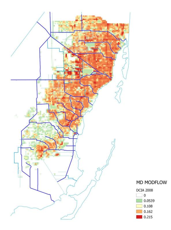
Figure 6. DCIA fractions for model grid cells in 2008.
