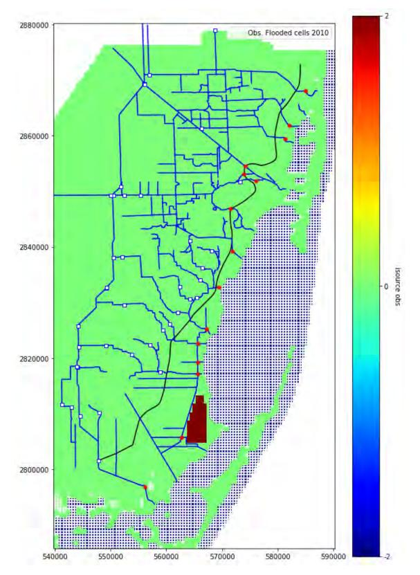
Figure 48. Freshwater/saltwater source (isource) for the 1996-2010 calibration run. Cells marked with white '+' are below the 2010 historical mean sea level at Virginia Key and their isource value is (for the most part) equal to -2 (blue). X and Y coordinates in meters, UTM17N, NAD83.
