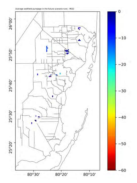
*Figure 55.* Average wellfield pumpage in the future scenario and sensitivity runs in MGD. Higher pumpage values are indicated by dark red colors (i.e. higher negative recharge).
