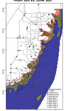
Difference in freshwater/saltwater interface HIGH SLR vs. LOW SLR
