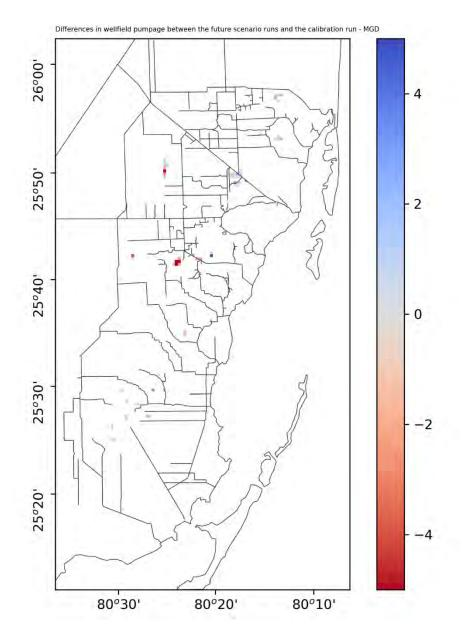
Figure 56. Differences in average wellfield pumpage in the future scenario and sensitivity runs minus the calibration run in MGD. Higher pumpage values in the future scenario runs are indicated by red colors (i.e. higher negative recharge). Differences range from -21 to +16 MGD at individual model cells, but -5 to +5 MGD range chosen for display purposes.
