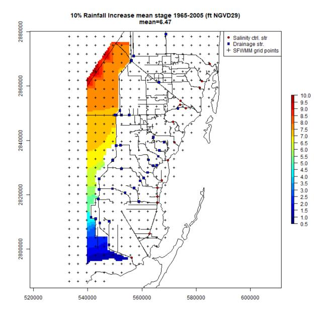
Figure 43. Average simulated stages for the 10% increased rainfall scenario (1965-2005). X and Y coordinates in meters, UTM17N, NAD83.
