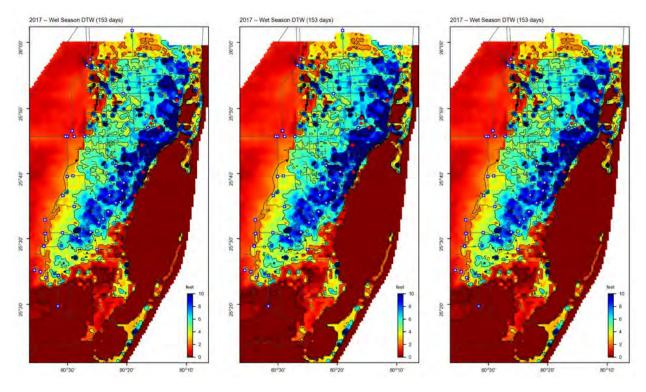
Figure 17. 2017 simulated average wet season depths to water in feet. Depths to water based on observed tide water level input (left), predicted tide without trend input (center), and predicted tide with added trend (right). Red dots are salinity control structures. White boxes with blue outlines are water supply/flood control structures.
