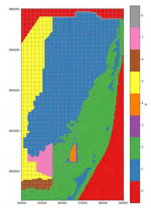
Figure 85. Boundary condition ids for Miami-Dade MODFLOW cells
