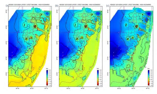
Figure 62. Simulated heads of High SLR scenario on (a) 12/31/2024, (b) 12/31/2039 and (c) 12/31/2054.
