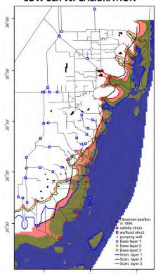
Difference in freshwater/saltwater interface LOW SLR vs. CALIBRATION
