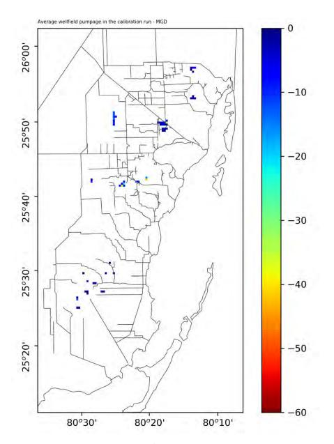
Figure 54. Average wellfield pumpage during the calibration/verification period (1996-2010) in MGD. Higher pumpage values are indicated by dark red colors (i.e. higher negative recharge).
