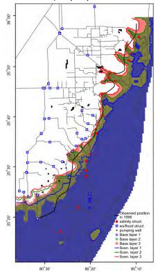
Difference in freshwater/saltwater interface (LOW SLR + HIST RAIN/RET) vs. LOW SLR
