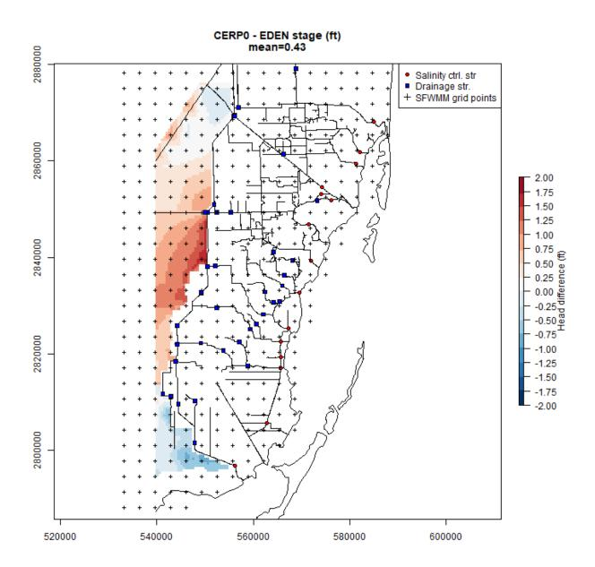
Figure 45. Differences between simulated stages in the CERPO scenario (1965-2005) and the EDEN dataset (1996-2010). X and Y coordinates in meters, UTM17N, NAD83.
