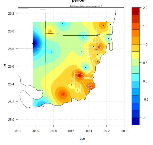
Figure 131. 50th percentile of adjusted DDF precipitation depths (inches) for the period centered in 2065 (2050-2079) minus DDF precipitation depths fit to observational data in the current baseline period (last 30 years up to 2005)  $(F_{m-padj.1} - F_{o-c})$  for 24-hour duration, 100-year return period.
