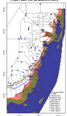
Difference in freshwater/saltwater interface LOW SLR + HIST RAIN/RET vs. CALIBRATION
