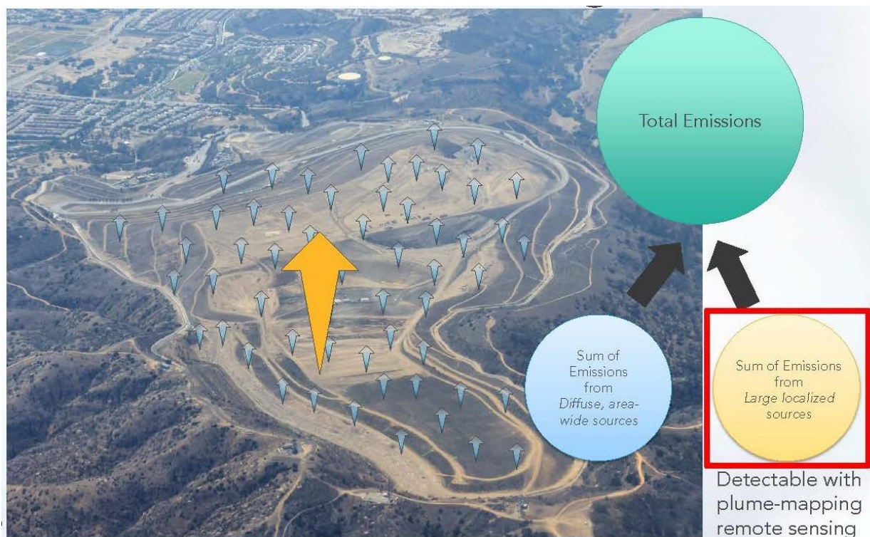
Point source emissions are represented by the large yellow arrow; area sources are represented by small blue arrows.
