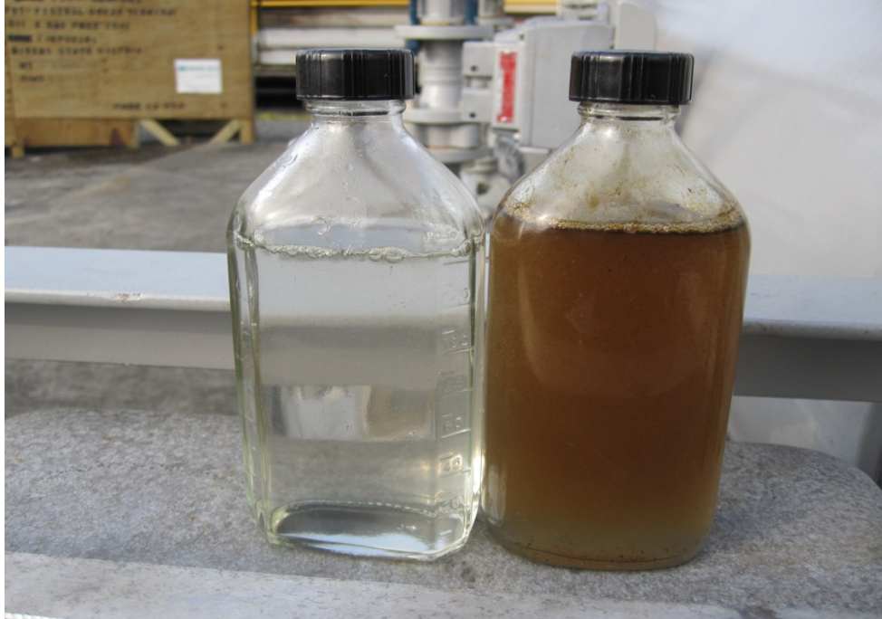
Figure 17: Inlet and Outlet Water Sample from Enviro-cell Unit with Higher Hydrocarbon Content in Produced Water.
