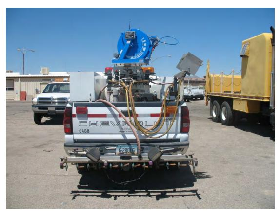
Photo 3. 4x4 3/4-ton truck with low boom sprayer.
