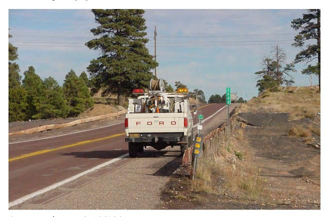
Photo 2. 4x4 3/4-ton truck with high boom sprayer.
