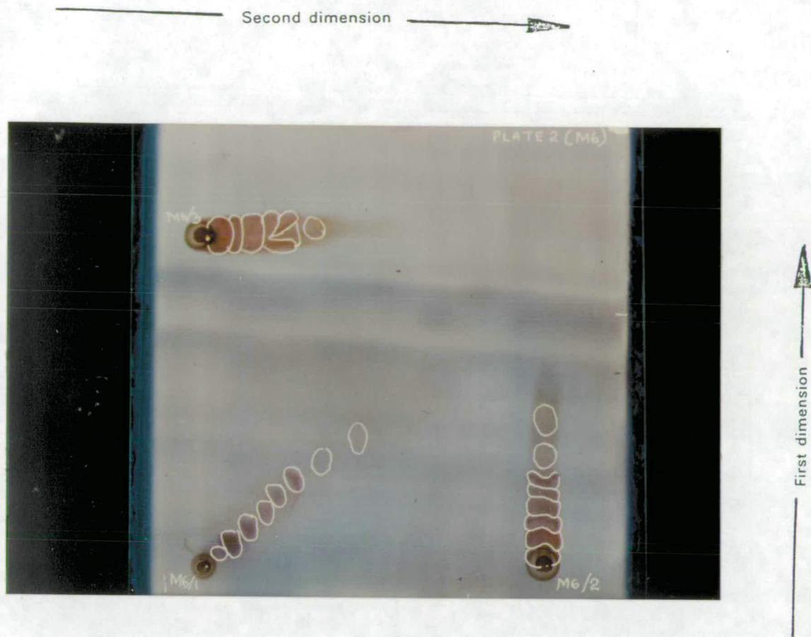
Fig:47 Two-dimensional TLC of free-amino acids extracted from larch sapwood
