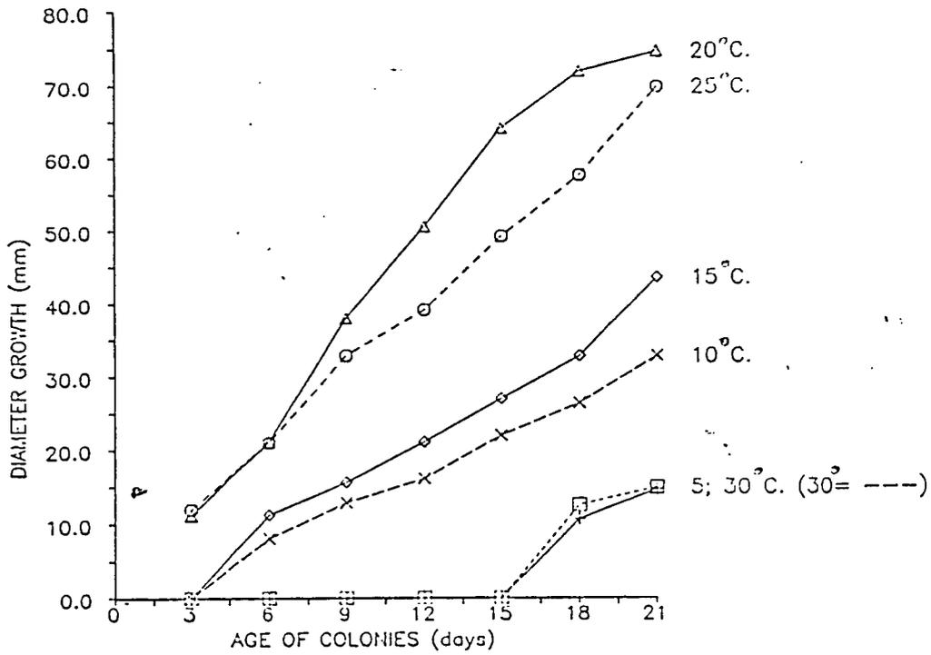
Fig:58 Effect of temperature on growth of *Ceratocystis piceae* on larch sapwood/agar meal.
