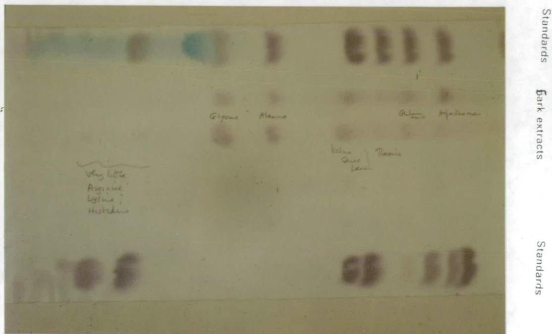
Fig:49 Separation of amino acids in larch bark extracts by High Voltage Electrophoresis (H.V.E.P.).
