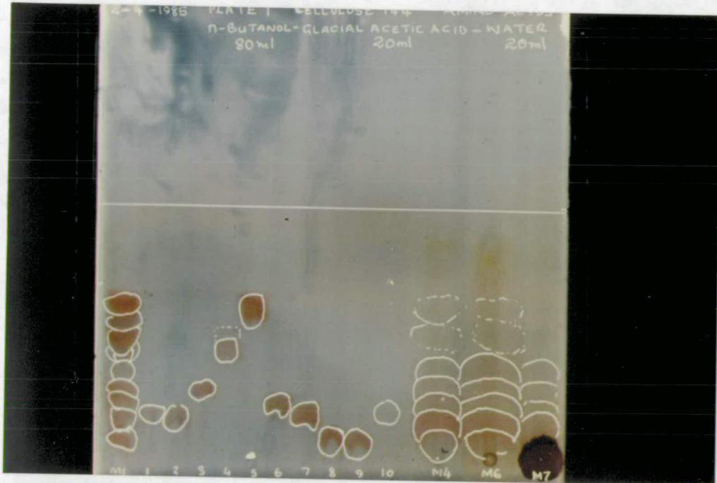
Fig:44 One-dimensional thin-layer chromatography (TLC) of larch inner bark free amino acids extract obtained by using cold 70% ethanol.
