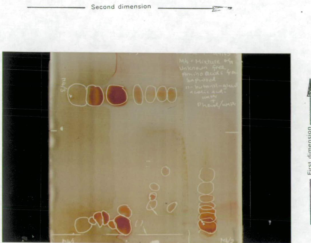
Fig:46 Two-dimensional TLC of free-amino acids extracted from larch sapwood.
