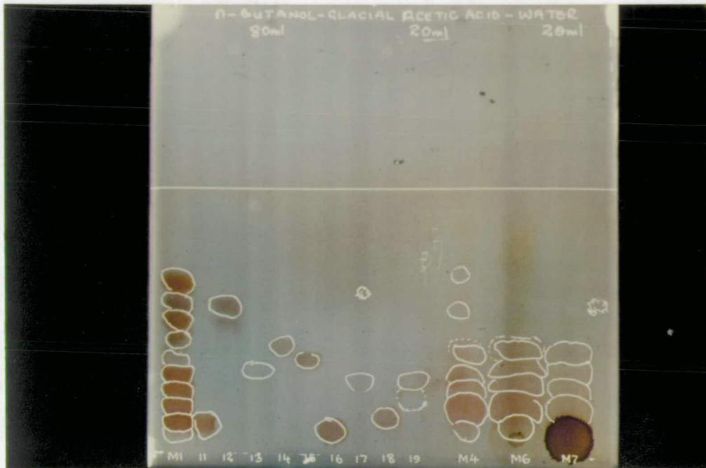
Fig:45 One-dimensional thin-layer chromatography (TLC) of larch inner bark free amino acids extract obtained by using cold 70% ethanol.
