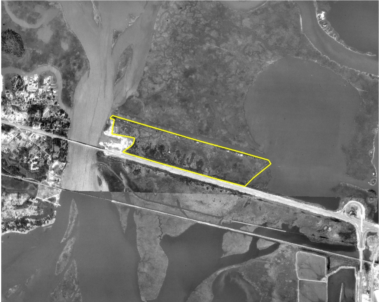
Figure E-8. Ingalls Restoration Site, MS. Example of marsh with moderate-low edge:area ratio. Only one edge of linear shoreline open to tidal flooding; length of shoreline is small relative to total area
