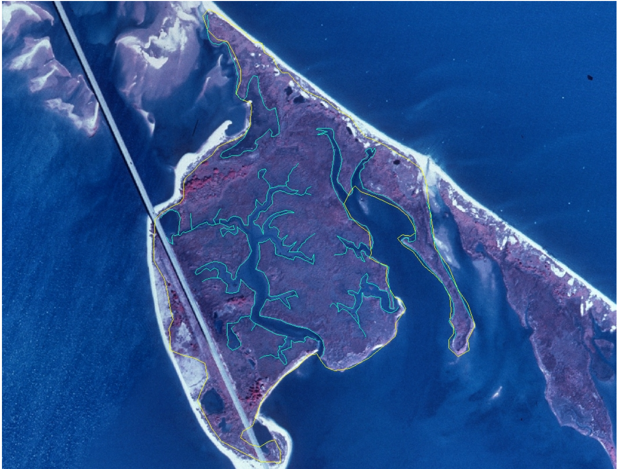
Figure E-1. Little Dauphin Island, AL. Example of marsh with high edge:area ratio. Note extensive tidal channel development with 1st-, 2nd-, and 3rd-order channels draining a large proportion of the total area of the WAA. WAA outlined in yellow. Tidally connected edge outlined in light blue.
