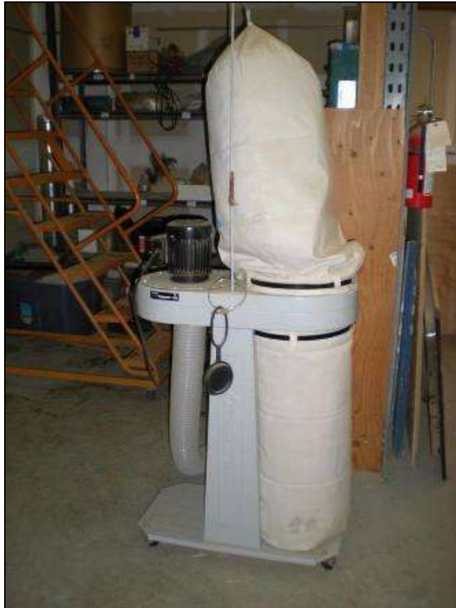
Figure 25. This Delta dust collector was used in conjunction with a Wall Mount air separator, in substitution of the canister vacuum that originally powered the air separator.
