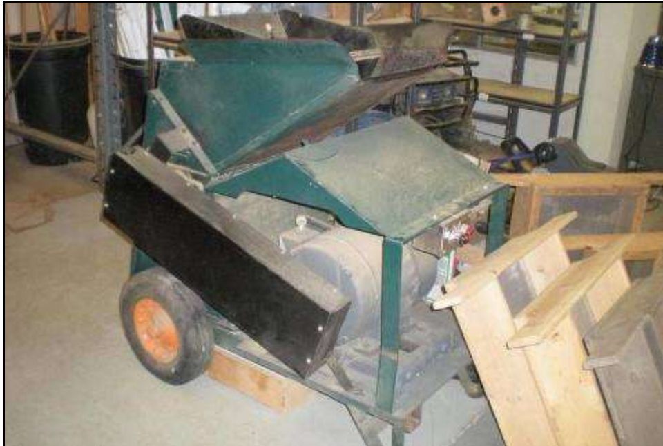
Figure 21. For the majority of the seed lots, a hammermill was used to reduce harvested plant material into a coarse but uniform mixture of seeds and chaff (e.g., pieces of branches, stems, leaves, fruits, and floral structures).
