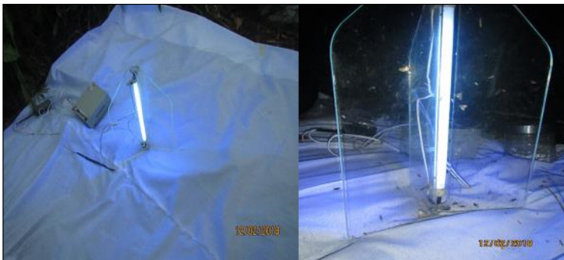
UV light trap powered by a 12V portable battery and set up on a 2 m x 2 m white sheet.
