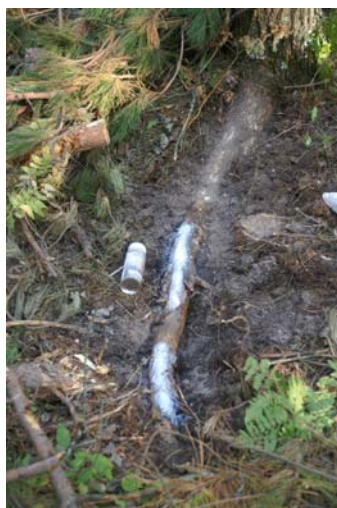
White pine root excavated to show injury along processor and forwarder trail. White paint has been sprayed on the root in the picture to the right in order to show portions of the root where logging equipment injured or removed bark.
